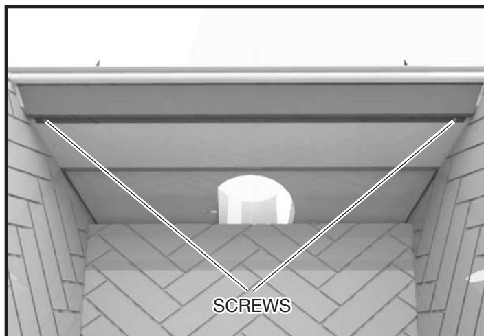
Figure 52: Side panel retainer location.
