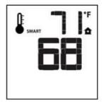
Figure 12: Smart flame function set low.
