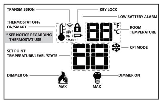
Figure 2: Proflame 2 LCD screen details.
