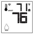
Figure 11: Smart flame function.
