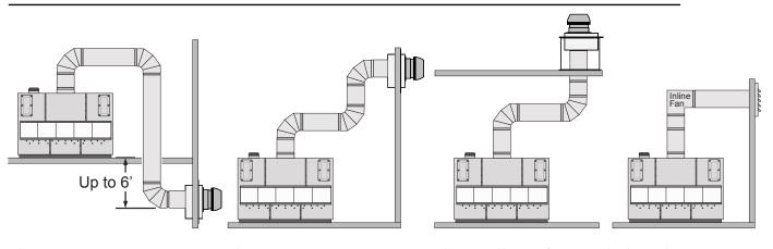
The Power Vent System on the DaVinci Custom Fireplace™ allows for nearly limitless venting configurations, even in the most challenging building situations.
