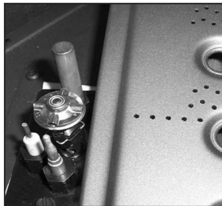
Figure 15: Ignitor assembly beside the burner.
