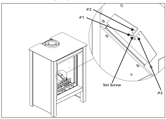
Figure 27: Installation of Air Restrictors
