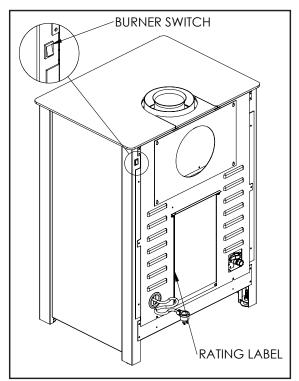
Figure 6. Burner Switch and Rating Plate
