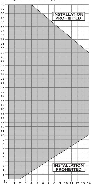
not exceed 44ft (13.4m). Any combination of rise and run can be used as long as it lays within the shaded area (a total of two (2) 90° elbows or four (4) 45° elbows can be used. In addition to what is shown, if a 90° elbow is used in the horizontal plane, 3 feet (91.4cm) must be subtracted from the allowable horizontal run (for each 45° elbow, 1½ feet must be subtracted).
