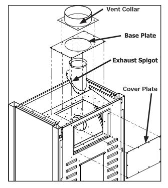
Figure 18. Vent Conversion - Step 2
