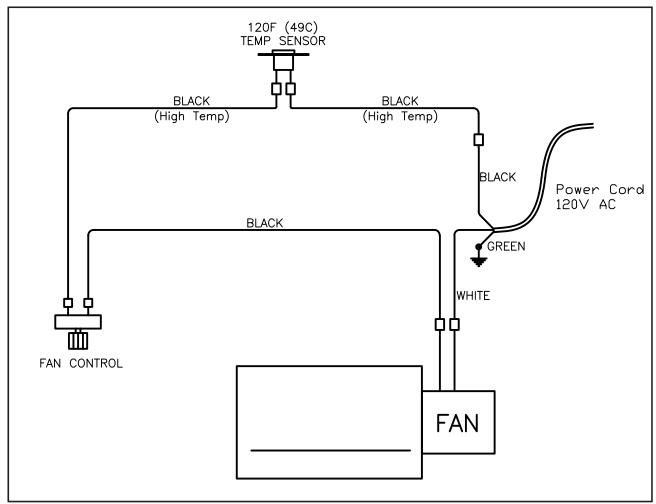
Figure 34: Fan wiring diagram.
