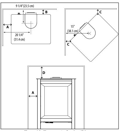
Figure 16. Clearance to Combustibles
