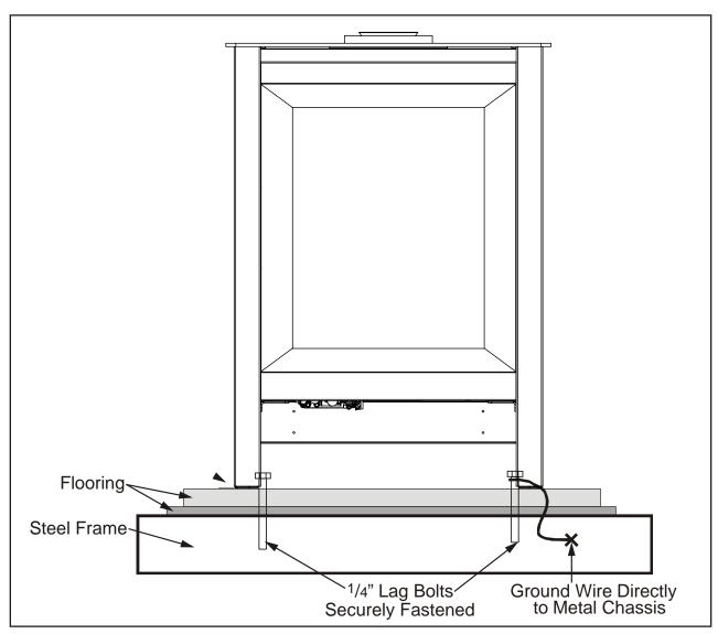
**Figure 24: Correct Mobile Home Installation**
