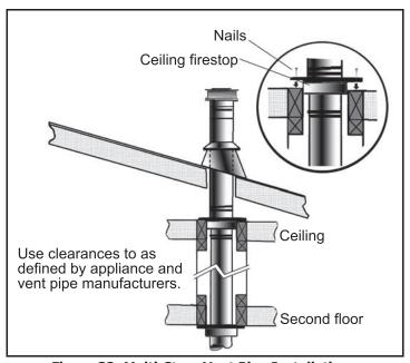
Figure 32: Multi-Story Vent Pipe Installation.
