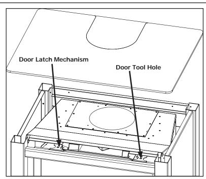
Figure 8. Top latches for glass door
