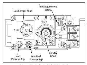
Figure 33: Fully Labeled Gas Valve.
