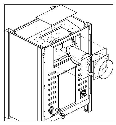
Figure 19. Vent Conversion - Step 3
