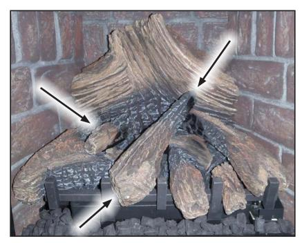
and left side log grate upright by locating the notch on the bottom side with the log grate cross bar. The top of the twig will rest on top of the far right curved twig. The last remaining straight twig gets intalled by locating the front in the crook of the far left y shaped twig and the back notch rests on the top edge of the ember bed.
