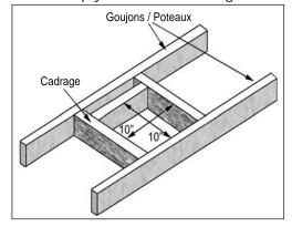
Figure 21. Vent Framing For Wall or Ceiling.
