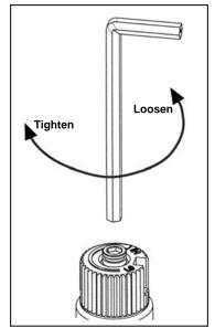
Figure 12: Removing valve screw.
