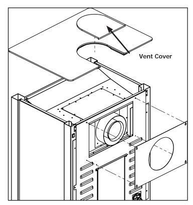
Figure 20. Vent Conversion - Step 4
