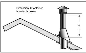
Figure 30: Height of Vertical Termination; Reference Table 7.
