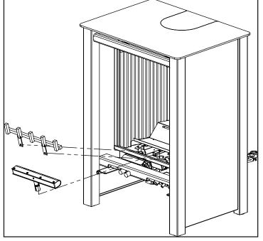
Figure 10. Removing Burner.
