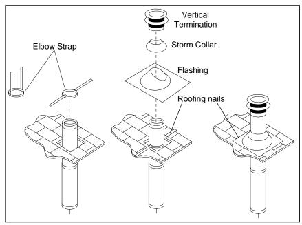
Figure 29. Vertical Vent Termination
