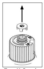
Figure 11: Removing valve cap.
