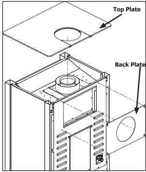
Figure 17. Vent Conversion - Step 1
