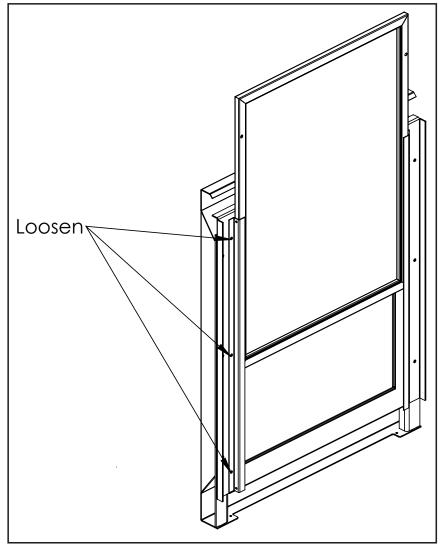
Figure 42. Safety Screen Removal
