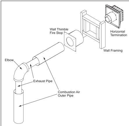
Figure 28. Horizontal Vent Termination
