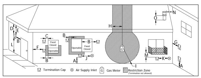
Figure 25. Vent Termination Restrictions, refer to Table 5.
