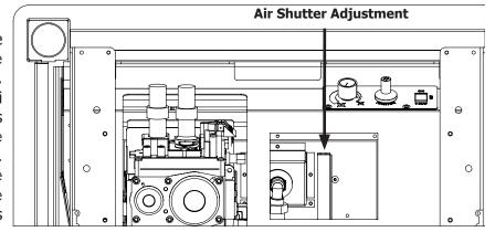
Figure 4. Air shutter adjustment lever.
