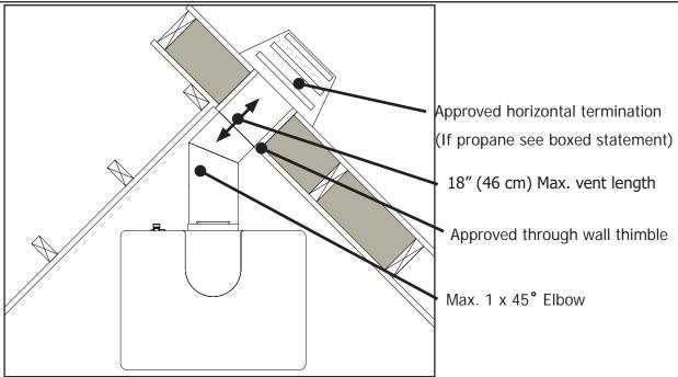
Figure 22. Corner Rear Vent - No Vertical Rise
