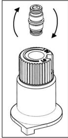
Figure C. Flip valve screw.
