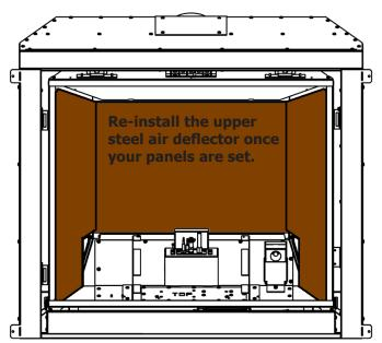
Figure 35. Liner panel position
