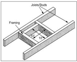
Figure 21. Vent Framing For Wall or Ceiling
