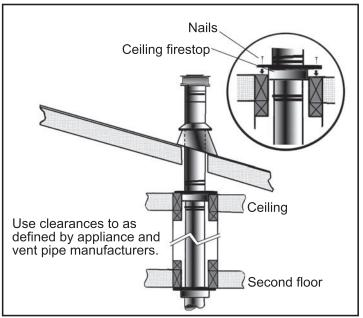
Figure 29: Multi-Story Vent Pipe Installation
