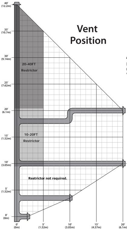
Any combination of rise and run can be used as long as it lays within the shaded area (a total of three (3) 90° elbows or six (6) 45° elbows can be used. In addition to what is shown, if a 90° elbow is used in the horizontal plane, 3 feet (91.4cm) must be subtracted from the allowable horizontal run (for each 45° elbow,  $1\frac{1}{2}$ feet must be subtracted).
