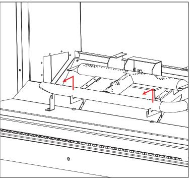
Figure 10. Removing Burner
