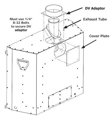
Figure 13. Vent Conversion - Step 1
