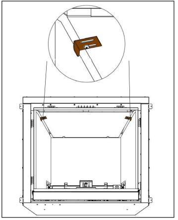
Figure 36. Liner panel retainers
