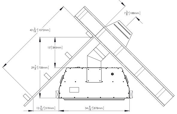
Figure 17A. Dimensions for a corner installation (Rear Vent)
