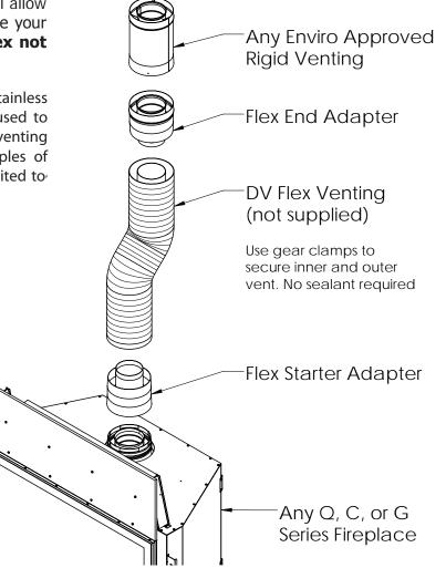
Figure 27. Flex Adapter Kit Install
