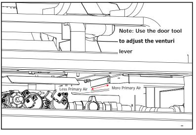
Figure 5. Air shutter adjustment lever
