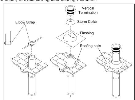
Figure 26A. Vertical Vent Termination
