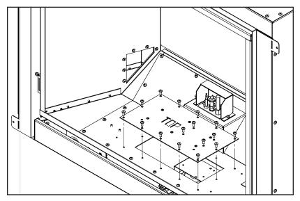
Figure 11. Removing Access Door
