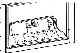
Figure 5: Valve Tray Removal
