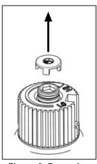
Figure A. Removing valve cap.
