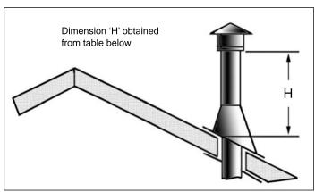
Figure 26B: Height of Vertical Termination; Reference Table 7
