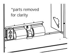
Figure 4: Fan Mounting
