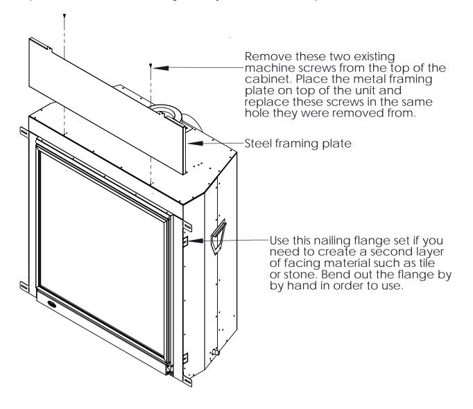
Figure 18A. Framing Plate Installation
