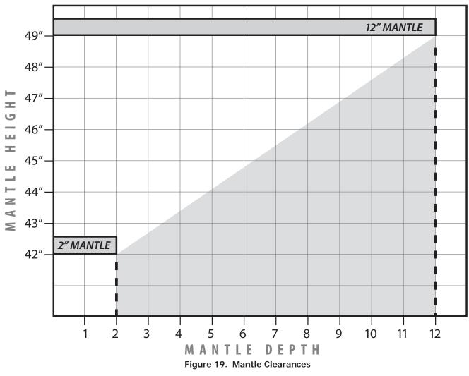
Note: Mantle height dimensions are based from the bottom of the appliance.
