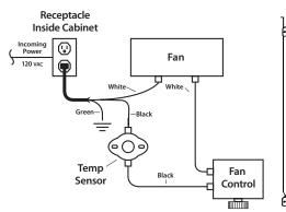
Figure 6: Fan Wiring
