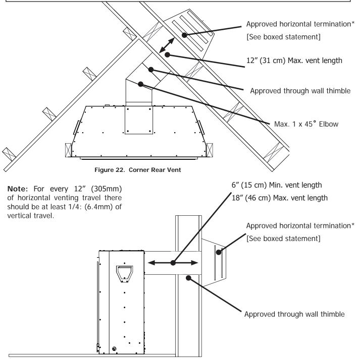
Figure 23. Flat to Wall Rear Vent
