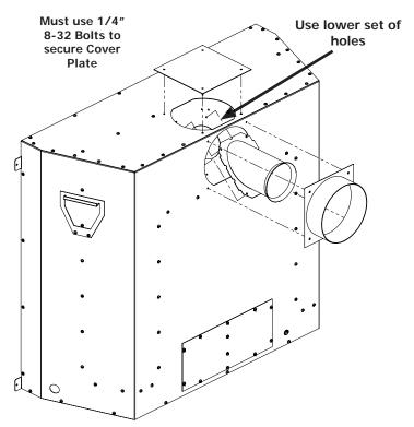
Figure 16. Vent Conversion - Step 2
