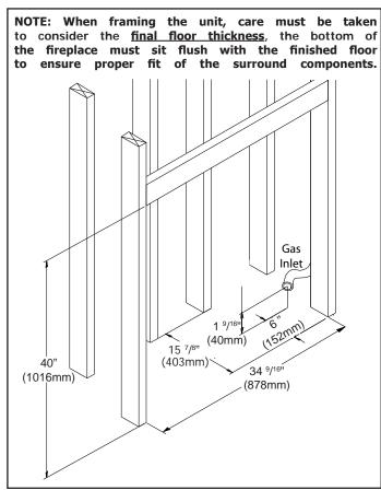
Figure 12. Framing Dimensions
