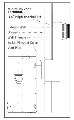
Figure 24. Possible Vent Configurations for Top Vent Only. Vertical and Horizontal Terminations
