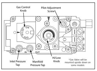
Figure 30: Fully Labeled Gas Valve.
