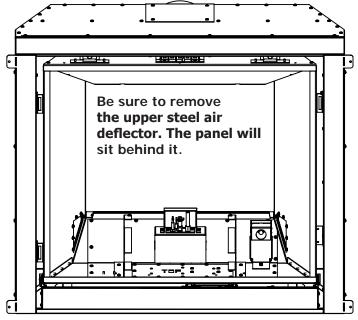
Figure 34. Firebox liner preperation
