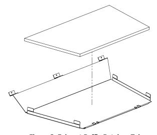
Figure 2. Exhaust Baffle Retainer Tabs
