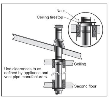
Figure 41B: Multi-Story Vent Pipe Installation
