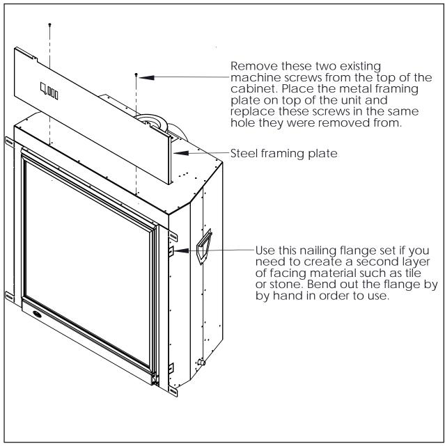
Figure 30. Framing Plate Installation
