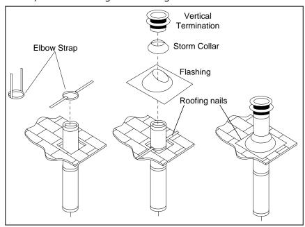
Figure 39. Vertical Vent Termination
