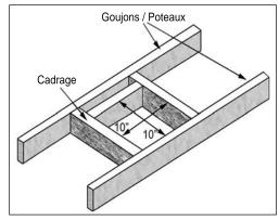
Figure 34. Vent Framing For Wall or Ceiling
