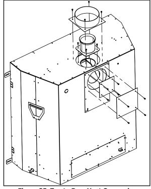
Figure 25. Top to Rear Vent Conversion
