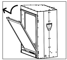
Figure 20. Door Removal Motion
