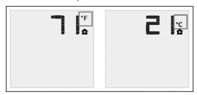
Figure 8: Remote Control Display in Farenheit and Celcius.
