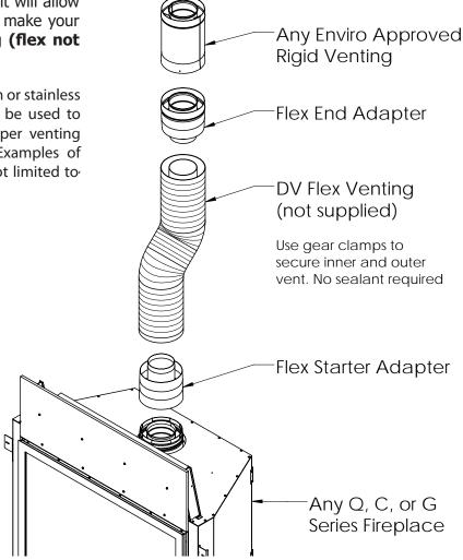
Figure 42. Flex Adapter Kit Install
