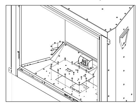
Figure 22. Removing Access Door
