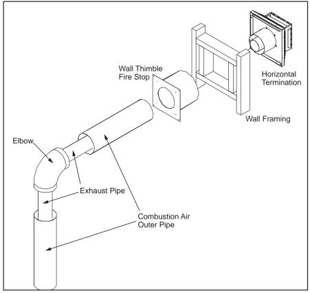
**Figure 38: Horizontal Vent Termination**
