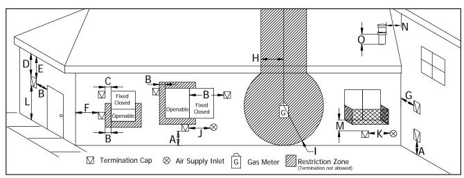
Figure 33. Vent Termination Restrictions, refer to Table 4
