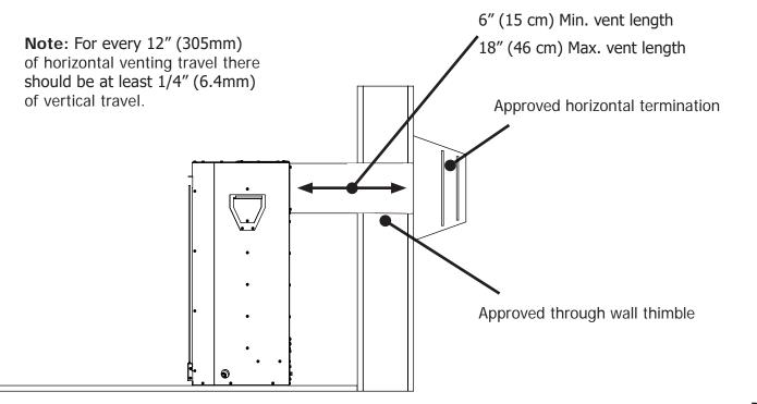
Figure 36: Parallel Vent Termination
