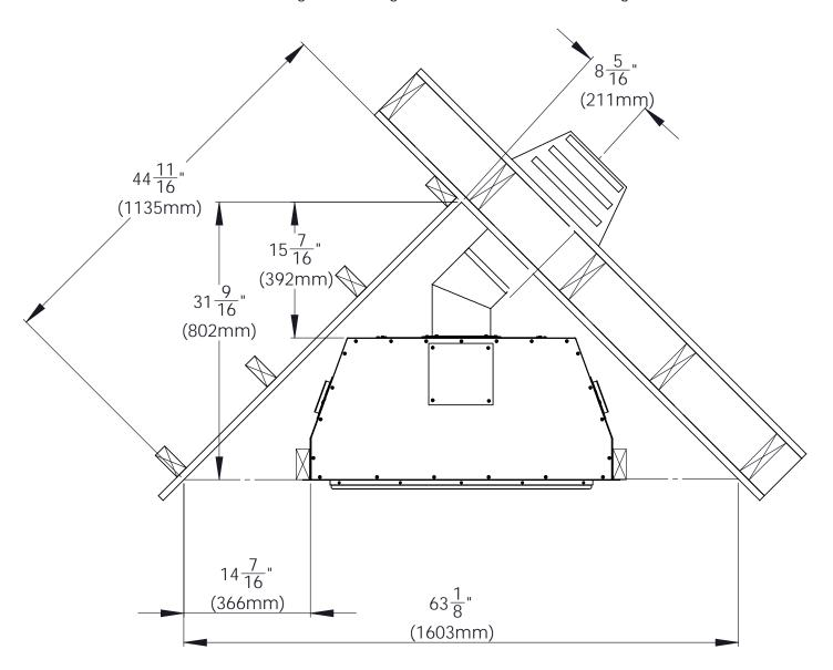
Figure 29. Dimensions for a Corner Installation
