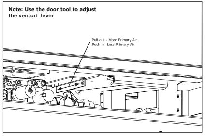
Figure 4. Air shutter adjustment lever.
