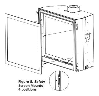
The door will occasionally need to be removed for installation of media, and cleaning of the Glass.
