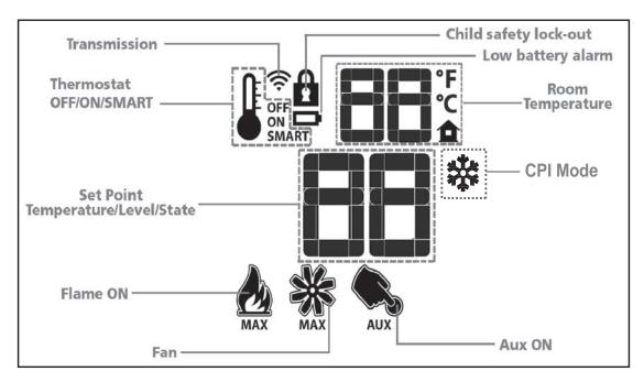
Figure 6: Proflame 2 Transmitter LCD Screen.
