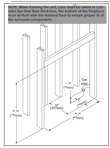
**Figure 28: Construction Framing Dimensions**
