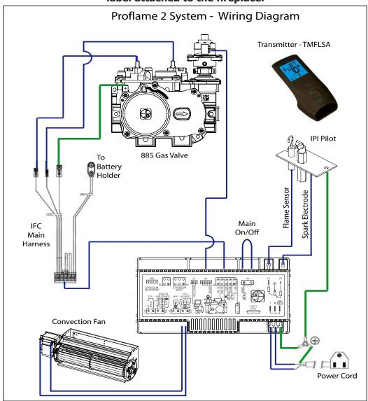
Figure 44: Wiring Diagram
