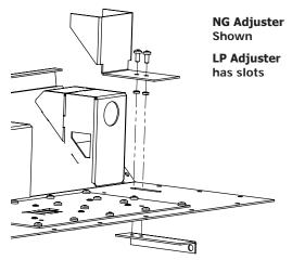
Figure A. Venturi Adjuster Replacement
