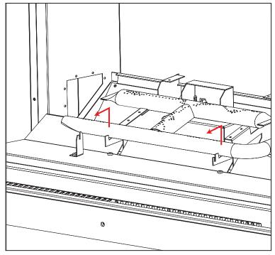
Figure 10. Removing Burner
