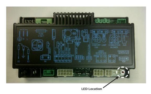
Figure 50: IFC LED Location
