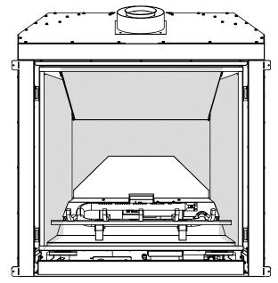
Figure 3. Liner panel position
