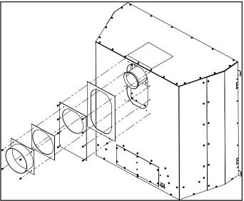
Figure 27A: Intake Block Off Plate Assembly Diagram
