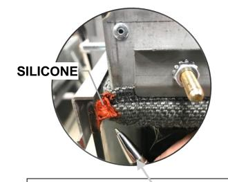
▲ IMPORTANT: Each corner must have a dab of high-temp silicone placed between the ball of the gasket and the corner glass. This will fully seal the firebox corners.
