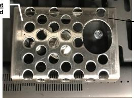
\*Pilot Shield should be visually inspected monthly for signs of deterioration due to flame exposure. Replace if necessary.
