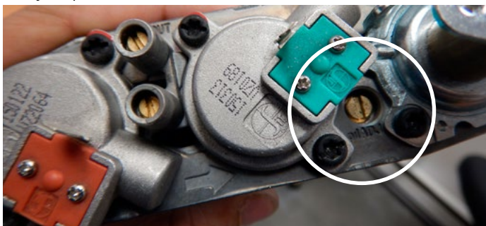
Figure 13.g Adjust pilot size
