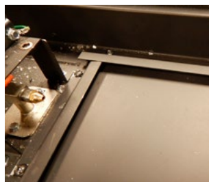
Figure 12.f Unscrewing brackets securing metal plate
