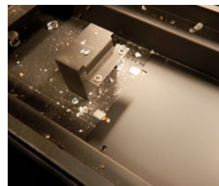
Figure 12.f Unscrewing brackets securing metal plate
