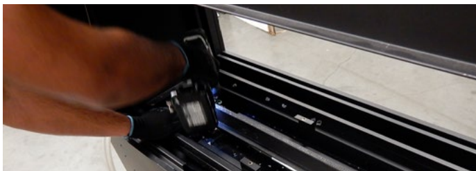
Figure 12.d Removing the Burner screws
