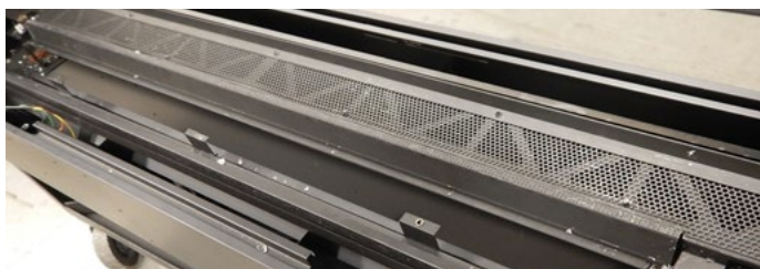
Figure 12.c Removing the media trays
