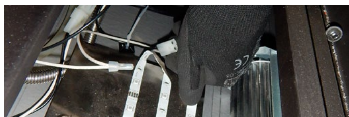
Figure 27.f Connect control board connector
