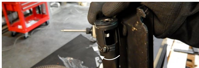
Figure 13.b Loosening the venturi
