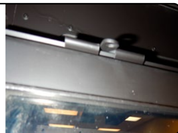
Figure 21.c Locate door latches
