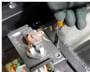
Figure 13.c Removing the orifice
