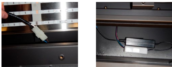
Figure 25.c Power LED receiver
