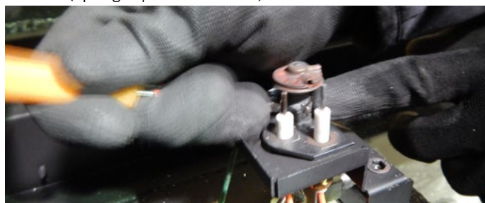
Figure 13.d Removing the spring clip
