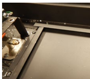
Figure 12.f Unscrewing brackets securing metal plate
