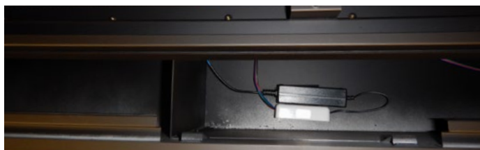
Figure 25. Secure LED receiver
