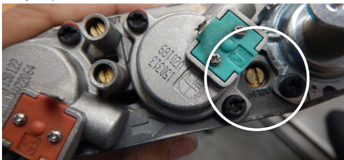
Figure 13.g Adjust pilot size
