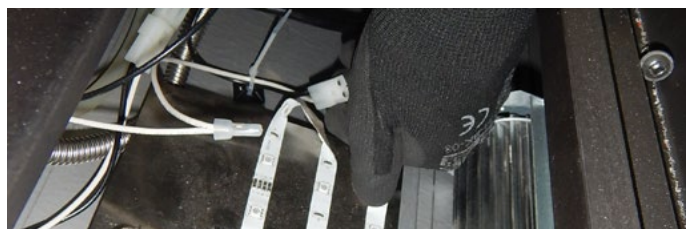
Figure 27.f Connect control board connector
