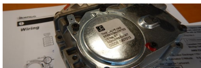
Figure 13.k Conversion label on valve
