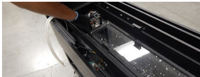
Figure 25.d Insert glass plate
