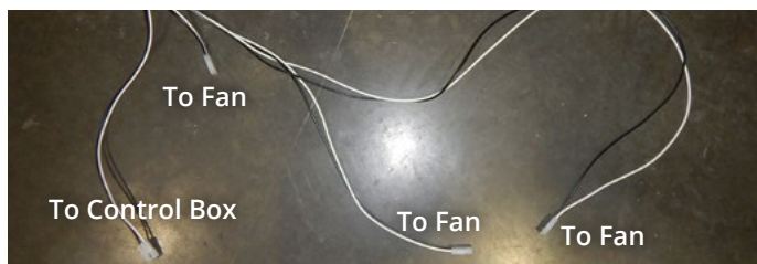
Figure 27.e Locate fan wiring harness
