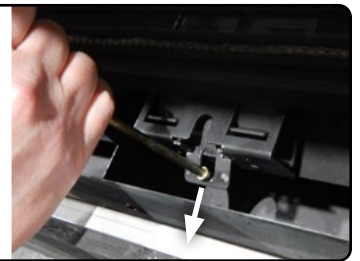
Figure 21.d Pull door latches
