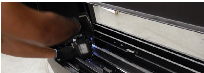
Figure 12.d Removing the Burner screws
