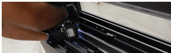
Figure 13. Removal of burner strip
