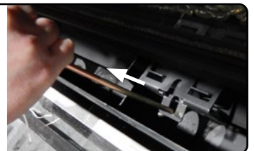
Figure 21.d Pull door latches
