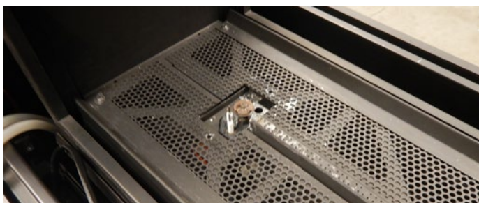
Figure 12. Removal of the pilot cover
