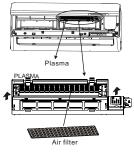
Hold the two partsof Plasma where are marked with f signal andlift it. Then you can open the coverof the the plasmaand remove the filter.
