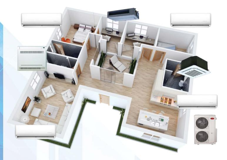
When you need to cool or heat more than one room, you don't have to install a separate system. You can choose our multi-zone models which will heat or cool many rooms by matching up to 5 indoor units to different outdoor units.
