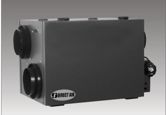
The PHRV200 series of Heat Recovery Ventilators (HRV) by Powrmatic. Incoming fresh outdoor air is filtered before it is heated by the stale outgoing air through a polypropylene heat recovery core. The HRV then distributes the preheated fresh filtered air throughout the home by direct ductwork installed specifically for the HRV or through the ductwork of a forced-air system.
