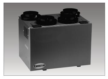
The PHRVR205 Heat Recovery Ventilators (HRV) by Powrmatic. Incoming fresh outdoor air is filtered before it is heated by the stale outgoing air through a polypropylene heat recovery core. The HRV then distributes the preheated fresh filtered air throughout the home by direct ductwork installed specifically for the HRV or through the ductwork of a forced-air system.
