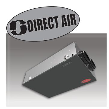
With a profile of only 8.75" high, the PHRVTE-120 is ideally suited for condos and apartments that have no mechanical room and where it must be located over a false ceiling. The PHRVTE-120 brings a continuous supply of fresh air into a home while exhausting an equal amount of contaminated air. The energy recovery core at the center of the unit transfers heat and moisture from the incoming air to the outgoing air that was cooled and dried by the building's air conditioner.
