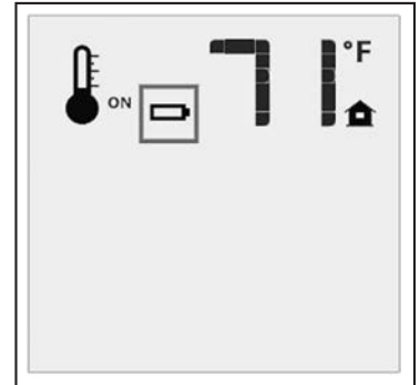
Figure 17: Low Battery Indicator.
