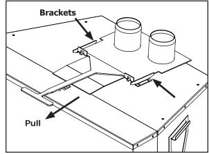
Figure 36: Vent Collar Plate Tool.
