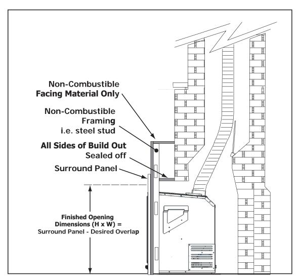
Figure 31: Installation with a non-combustible build out.
