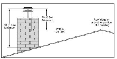
Figure 34: Roof Clearances.
