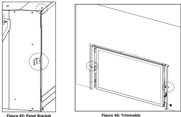
Figure 45: Panel Bracket Installed and Pin Location
