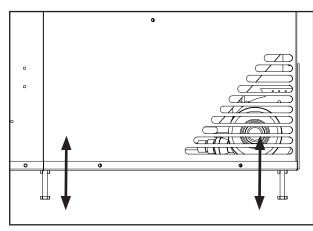
Figure 37: Levelling Legs Position.
