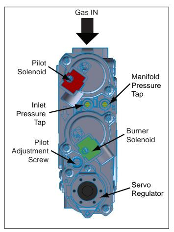
Figure 40: Fully Labeled Gas Valve.
