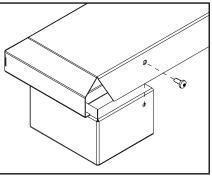
Figure 43: Installing Base Shelf onto Riser.
