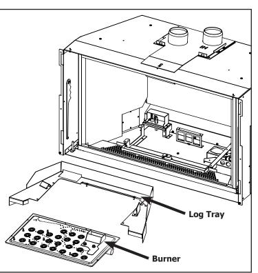
Figure 24: Burner Removal.
