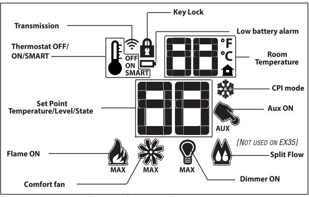
Figure 6: Proflame 2 Transmitter LCD Screen.
