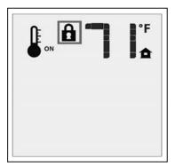
Figure 18: Remote Control Locked.
