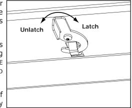
Figure 35: Vent Collar Plate Latch.
