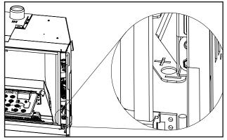
Figure 4: Adjusting the venturi air setting.
