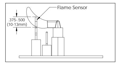
Figure 41: Proper Pilot Flame.
