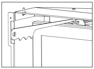
Figure 22: Door Latch Release.
