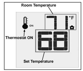
Figure 9: Remote Control Displays Set Temperature.
