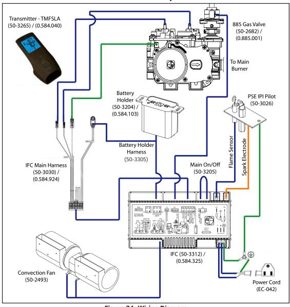
Figure 34: Wiring Diagram.
