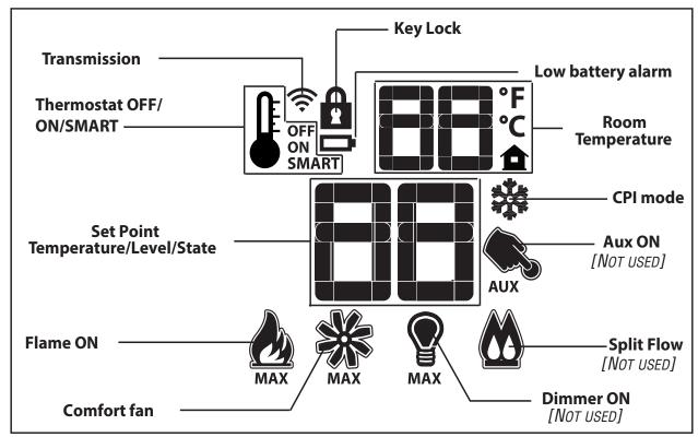
Figure 6: Proflame 2 Transmitter LCD Screen.
