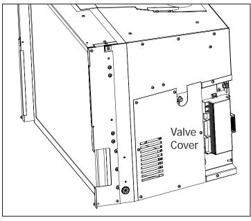
Figure 21: Valve Cover Location
