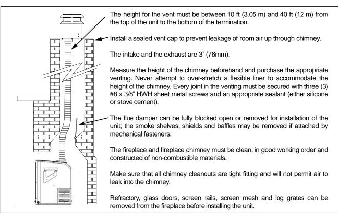
Figure 26: Installation of E44
