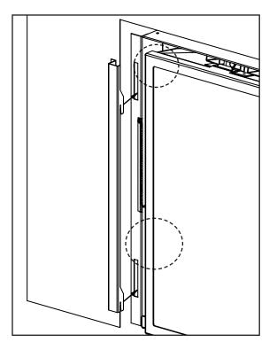
Figure 41: Panel Slot and Hook Locations
