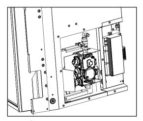
Figure 36: Gas valve with cover removed
