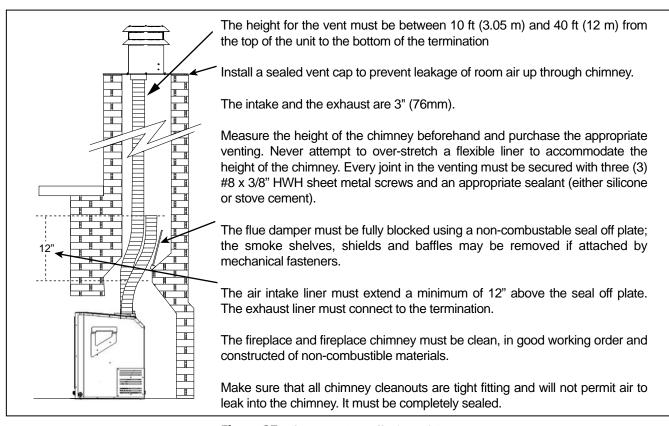
Figure 27: Alternate Installation of E44
