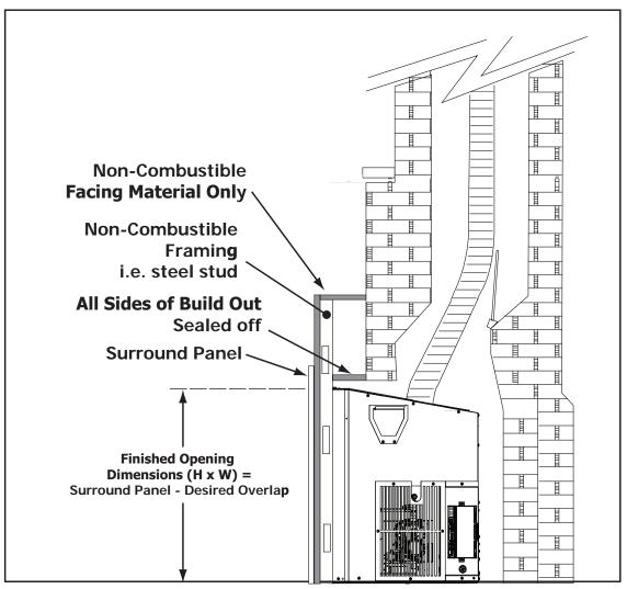
Figure 25: Installation with a non-combustible build out.
