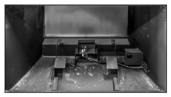
Figure 52: The rear liner can now be removed. Use a vacuum to clean up the bare firebox if needed.
