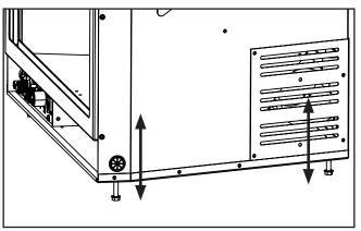
Figure 32: Levelling legs position.
