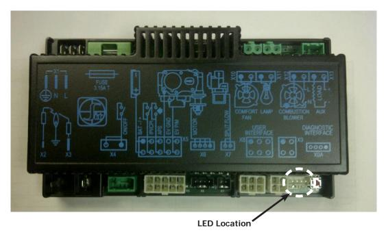
Figure 63: IFC LED Location
