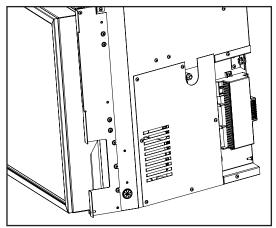
Figure 35: Gas connection location
