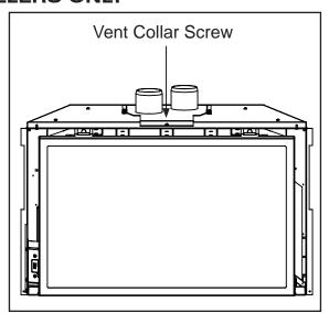
Figure 31: Vent Collar Plate Screw Location.
