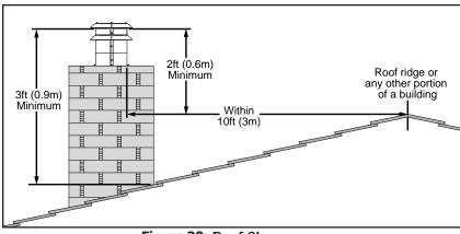
Figure 30: Roof Clearances.
