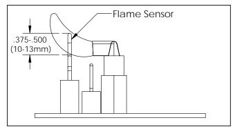
Figure 38: Proper Pilot Flame.
