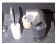
Figure 23: Proper Pilot Position
