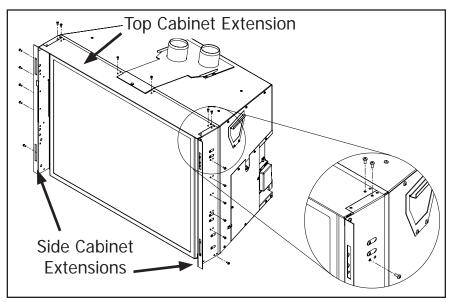
**Figure 43: Removing Extension Screws**
