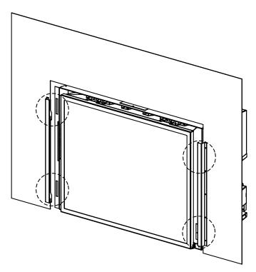
Figure 42: Trimmable Panel Installed
