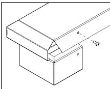
Figure 40: Installing Base Shelf onto Riser.
