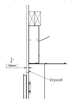
**Standard Extended Install:** Using the supplied long finishing edge, **non-combustible** material may be layered on top of the supplied Noncombustible board. Supplied board not needed for thick **non-combustible** finishes like rock.
