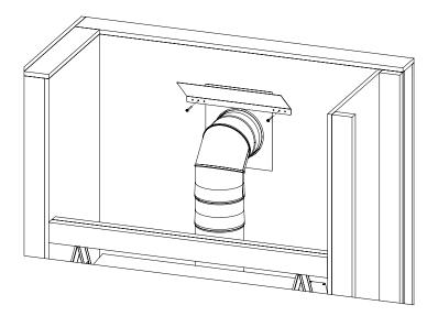
Figure 30: Rear Heat Shield
