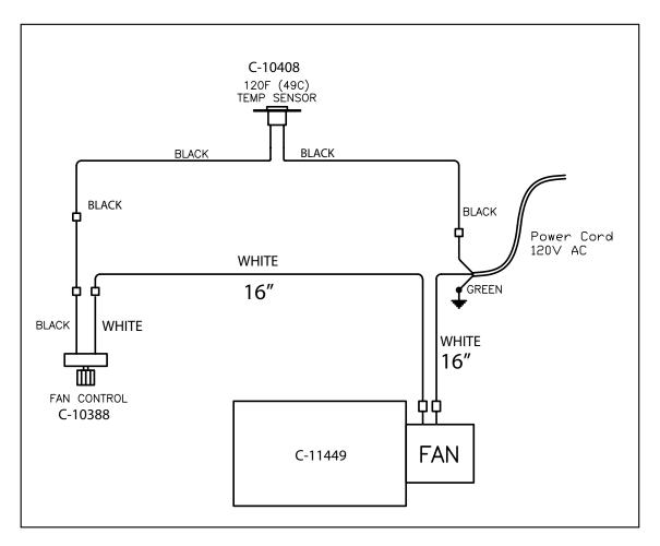
Figure 65: Convection Fan Wiring Diagram
