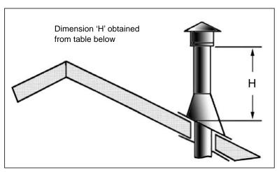
Figure 60: Height of Vertical Termination; Reference Table 7
