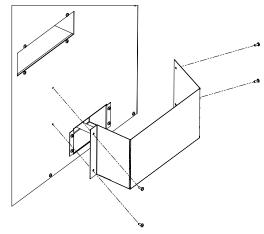
**Figure 19: Cabinet Holster Removal**
