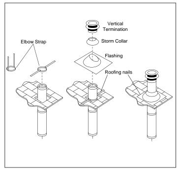
**Figure 59. Vertical Vent Termination**
