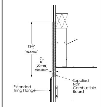
Cool Surface System Extended Install: Using the supplied long finishing edge, combustible material may be layered on top of the supplied Non-combustible board. Supplied board is not needed for thicker combustible finishes.
