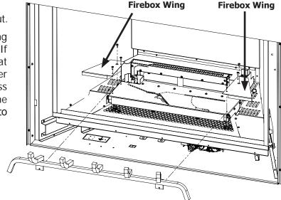
Figure 10. Front Burner Removal
