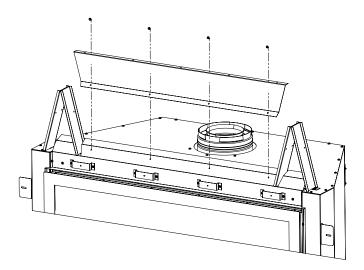
Figure 24: Heat Shield Support Install
