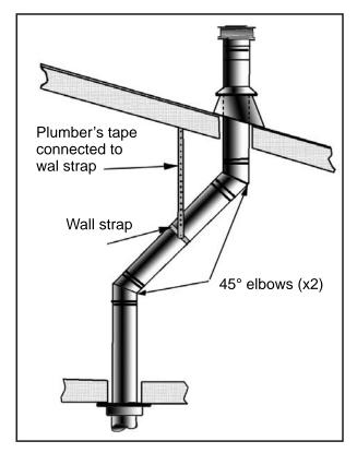
Figure 61: Multi-Story Vent Pipe Installation
