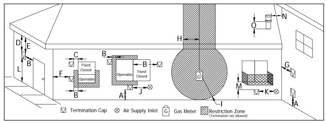
Figure 52. Vent Termination Restrictions, refer to Table 3
