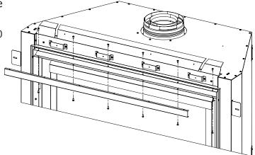
**Figure 32: Front Cover Removal**
