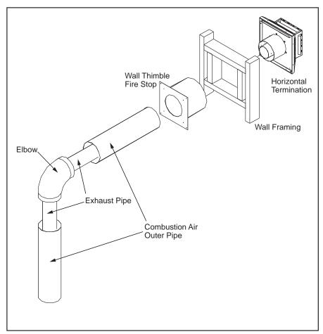
Figure 58. Horizontal Vent Termination
