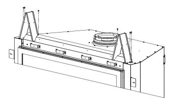
Figure 23: Top Standoff Install
