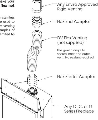
Figure 48. Flex Adapter Kit Install
