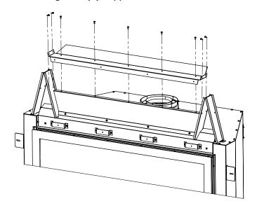
Figure 25: Standoff Brace Install
