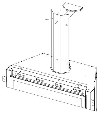
Figure 29: Vent Shields
