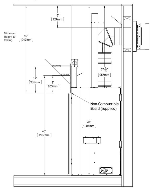
Figure 43: Flat Wall Installation
