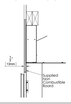
**Cool Surface System (CSS) Install:** Image shows the short finishing edge, **combustible** can be brought right down to the finishing edge.
