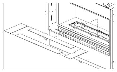
Figure 62: Burner Bezel Placement
