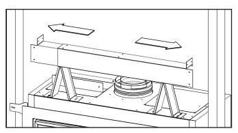
Figure 28: Steel Stud Placement
