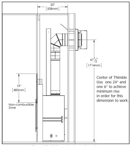
Figure 33: Minimum Horizontal Venting
