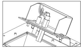
Figure 25: Flame Sensor Coverage
