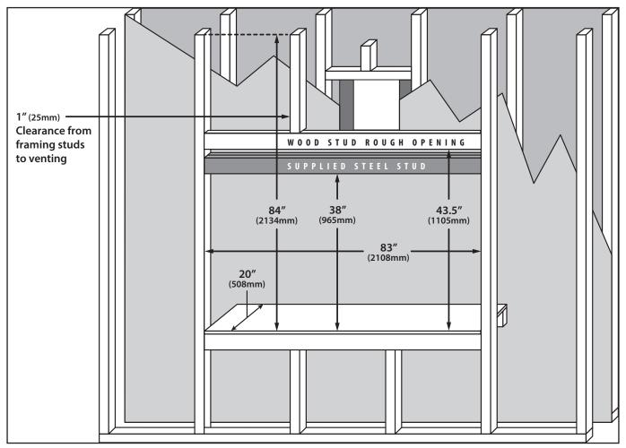
**Figure 31: Construction Framing Dimensions**
