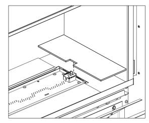
Figure 63: Bezel Placement Around Pilot
