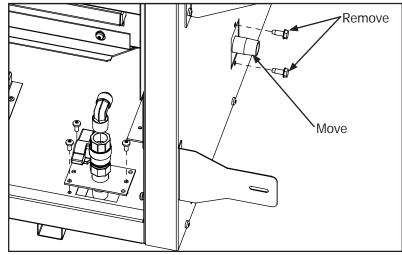
Figure 32: Alternate Gas Inlet Location
