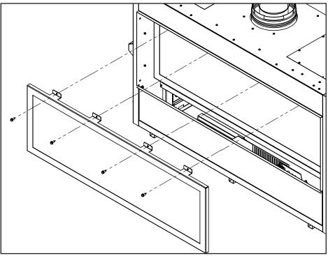
Figure 18: Door Removal Motion
