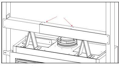
Figure 29: Steel Stud Attachment
