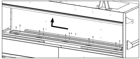
Figure 19: Removing Burner
