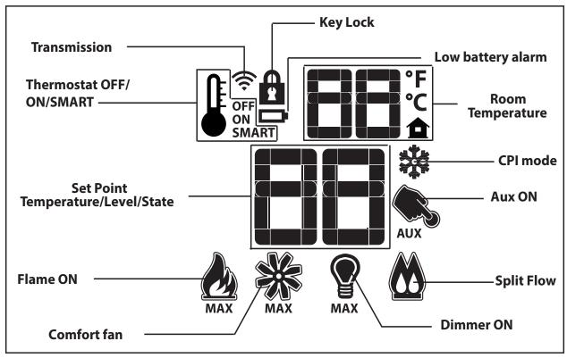
Figure 5: Proflame 2 Transmitter LCD Screen.
