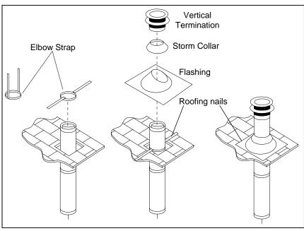
Figure 53: Vertical Vent Termination
