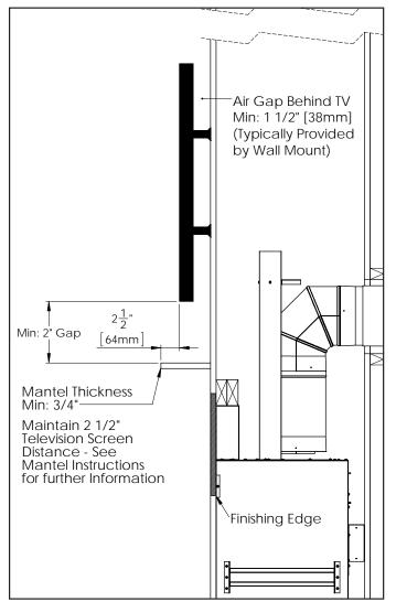
Figure 45: Minimum TV Install Clearances
