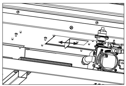
Figure 3: Air shutter adjustment lever
