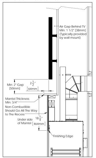
Figure 46: Recess Minimum TV Install Clearances
