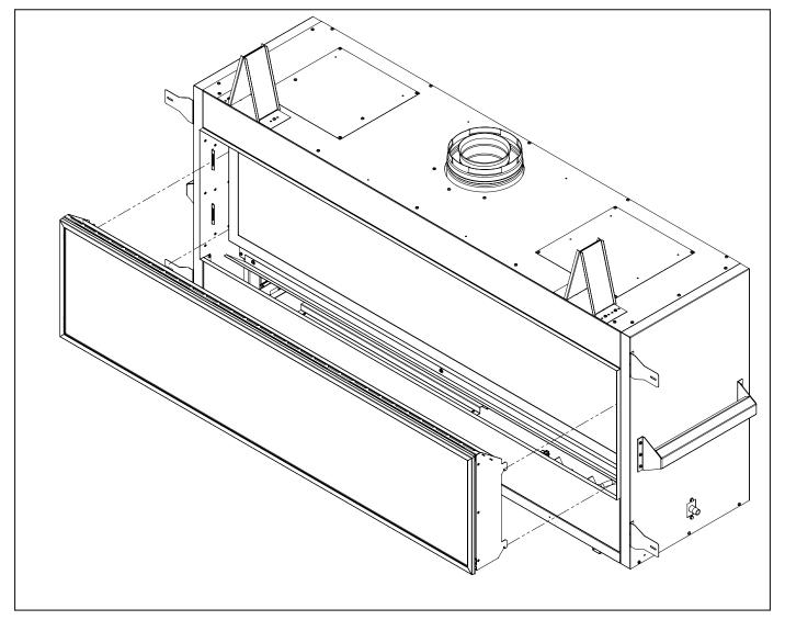
Figure 17: Safety Screen Removal
