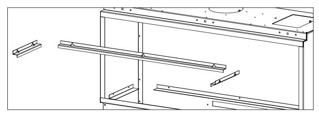
Figure 65: Panel Installation
