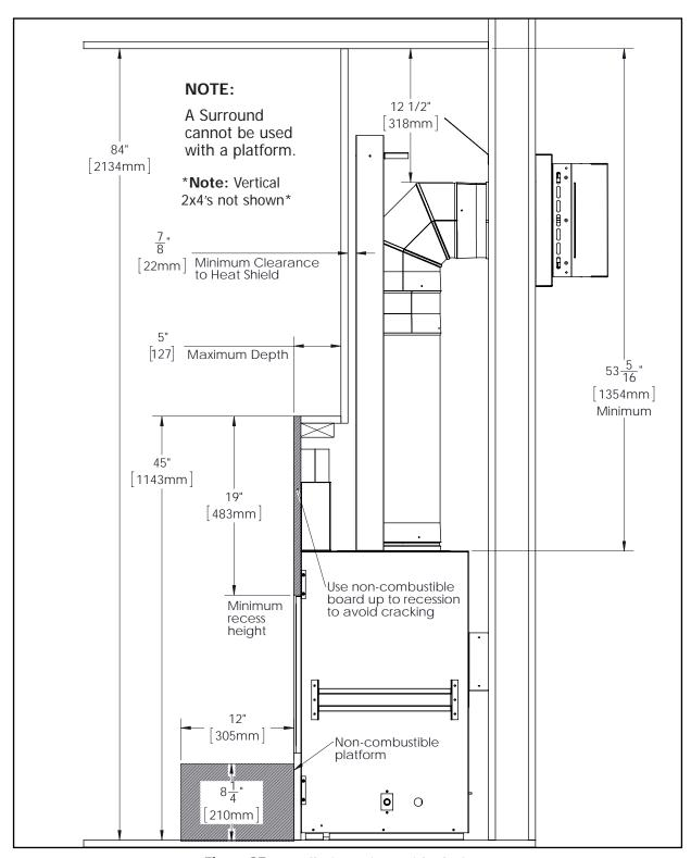
Figure 37: Install Dimensions with Platform
