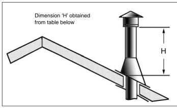
Figure 54: Height of Vertical Termination; Reference
