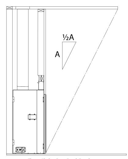
**Figure 42: Overhang Depth Requirements**
