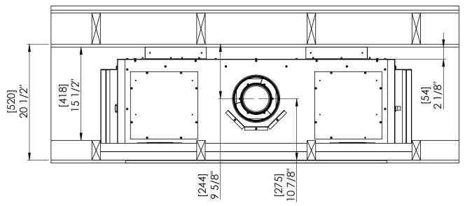
Figure 41: Dimensions for a Vertical Installation
