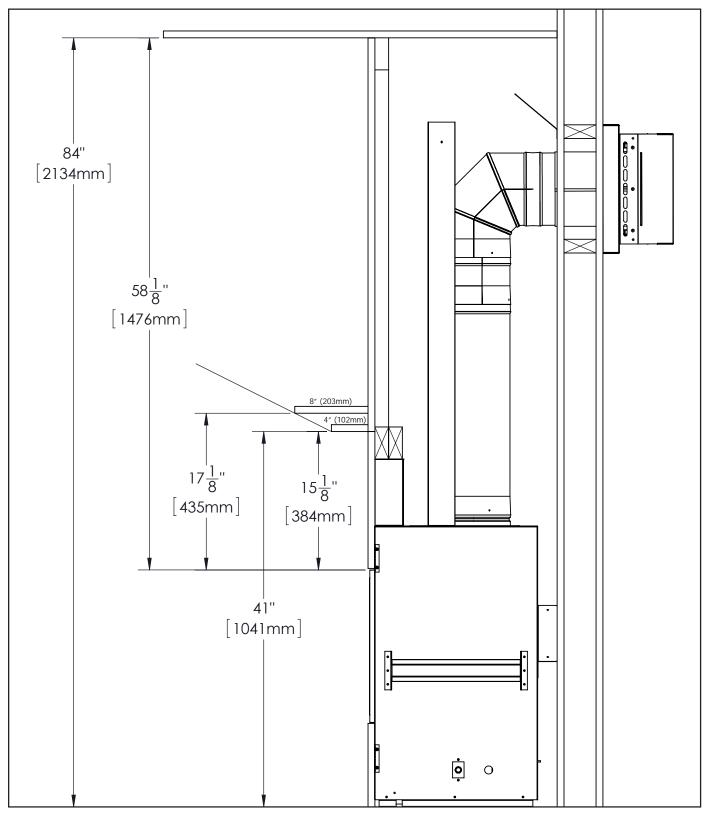
Figure 35: Install Dimensions with Mantel
