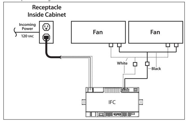
Figure 60: C72I Fan Kit Wiring Diagram. See 50-4173 instruction manual for C72ID wiring diagram
