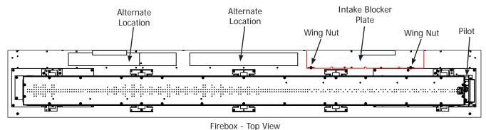
Figure 51: Intake Blocker Plate
