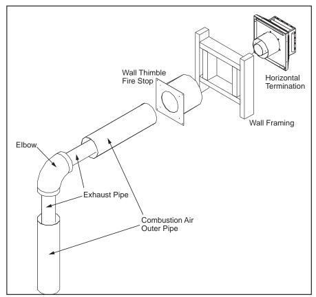
Figure 52: Horizontal Vent Termination
