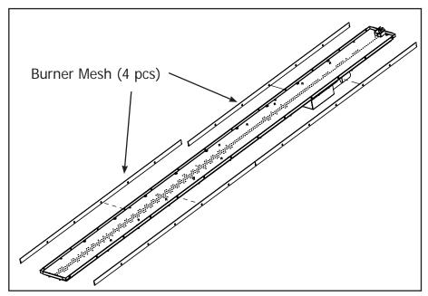
Figure 24: Burner Mesh Removal (LP ONLY)
