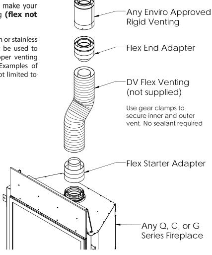
Figure 43: Flex Adapter Kit Install
