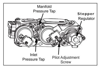
Figure 57: Fully Labeled Gas Valve. See Dexen User Manual for C72ID valve details
