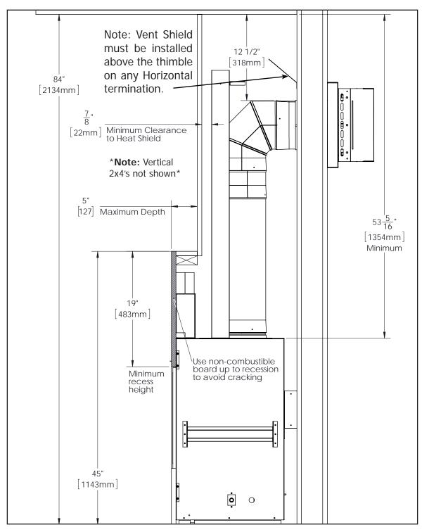
Figure 36: Install Dimensions with Recess
