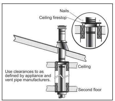
Figure 56: Multi-Story Vent Pipe Installation
