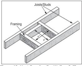
Figure 48: Vent Framing For Wall or Ceiling
