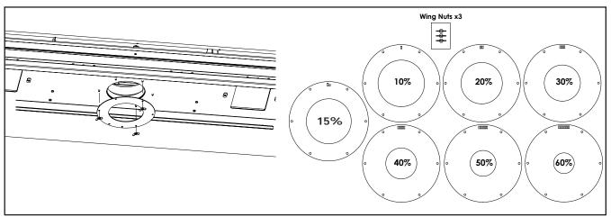
Figure 50: Restrictor Install and Ring Set
