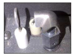
Figure 23: Proper Pilot Position
