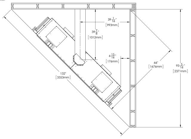
Figure 38: Dimensions for a Corner Installation
