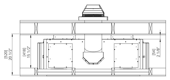
Figure 40: Dimensions for a Horizontal Installation
