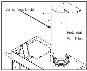
Figure 39: Vent Shielding Install
