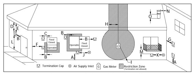
Figure 60: Vent Termination Restrictions, refer to Table 2
