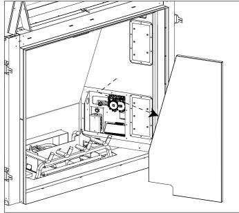
Figure 19: Right Liner Removal
