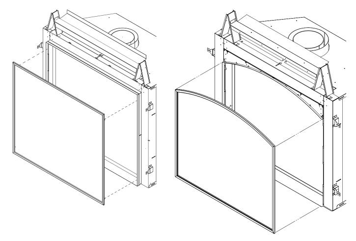
Figure 4: Safety Screen Removal (U441 and U441-A models)
