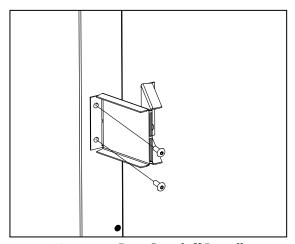
Figure 32: Rear Standoff Install
