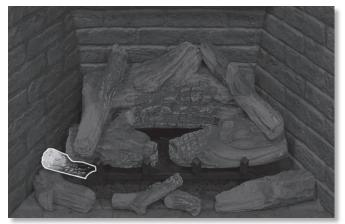
Figure 87: Log Set Installation - Step 10
