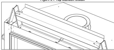
Figure 30: Top Standoff Support Install
