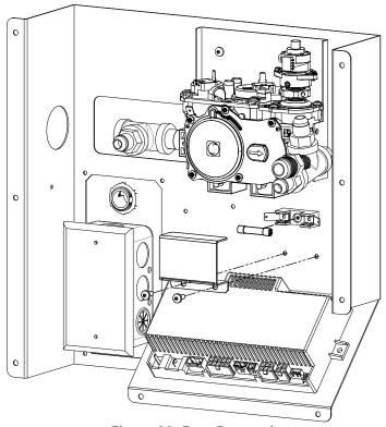
Figure 20: Fuse Removal
