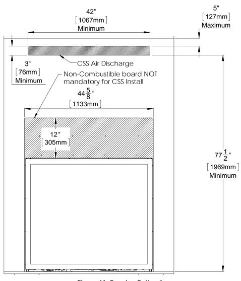
**Note:** If you wish to construct the CSS air discharge part way up a tall wall then it is essential to build a false ceiling inside the chase at the desired height to direct the rising heat out of the gap.
