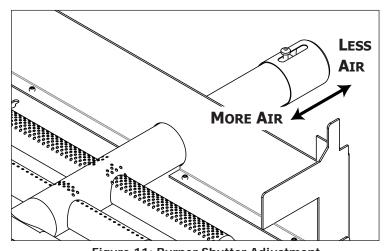
Figure 11: Burner Shutter Adjustment
