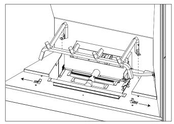
Figure 8: Log Grate Removal
