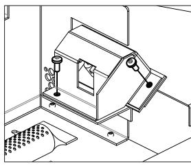
Figure 23: Pilot Shield Removal
