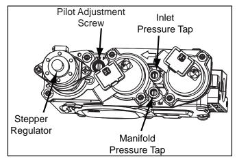
Figure 74: Fully Labeled Gas Valve.
