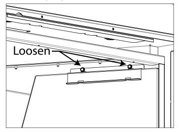
Figure 18: Liner Retainer Removal
