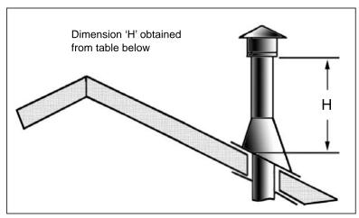
Figure 71: Height of Vertical Termination; Reference Table 8
