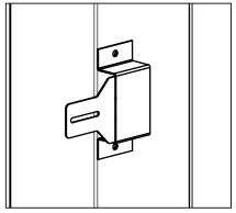
Figure 26: Nailing Flange Flat
