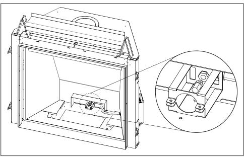
Figure 22: Orifice Location
