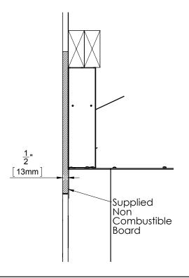
**Cool Surface System (CSS) Install:** Image shows how **combustible facing** can be brought right down to the finishing edge.
