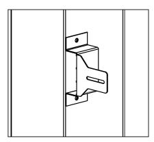
Figure 27: Nailing Flange Assembled
