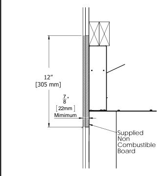
Cool Surface System Extended Install: By adjusting the cabinet back, combustible material may be layered on top of the supplied Non-combustible board. Supplied board is not needed for thicker combustible finishes.
