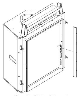
Figure 16: Side Panel Removal
