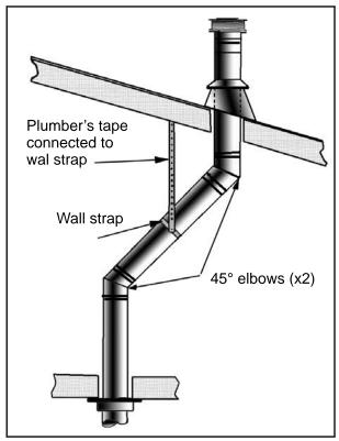
Figure 72: Multi-Story Vent Pipe Installation
