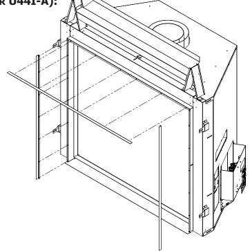
Figure 33: Finishing Edge Removal / Installation
