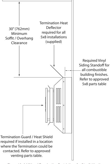
Figure 62: Additional Termination Restrictions for 5" x 8" Venting
