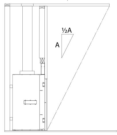
Figure 52: Overhang Depth Requirements
