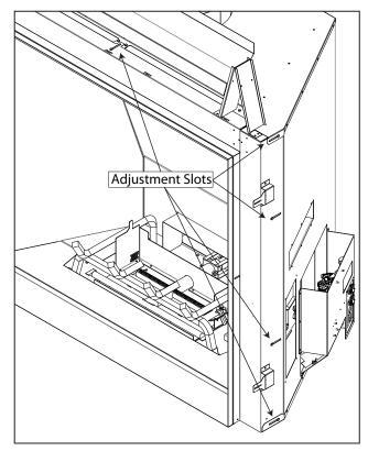
Figure 36: Framing Depth Adjustment
