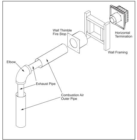
Figure 69: Horizontal Vent Termination
