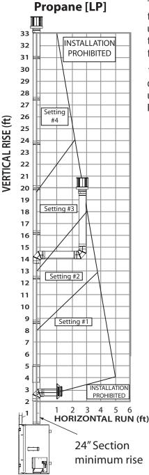
The following diagrams show the range of venting options using either vertical or horizontal terminations. Any layout within the shaded area is acceptable.
