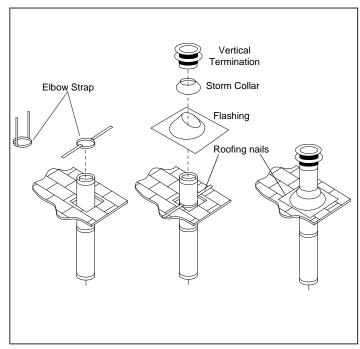
**Figure 70: Vertical Vent Termination**
