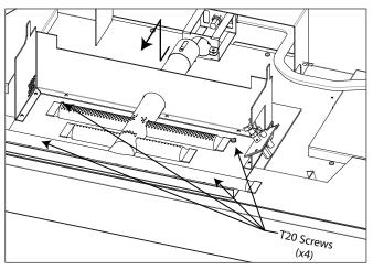
Figure 10: Log Burner Removal
