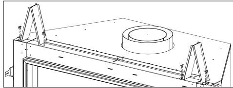
Figure 29: Top Standoff Install
