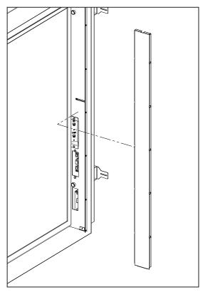
Figure 35: Side Cover Removal
