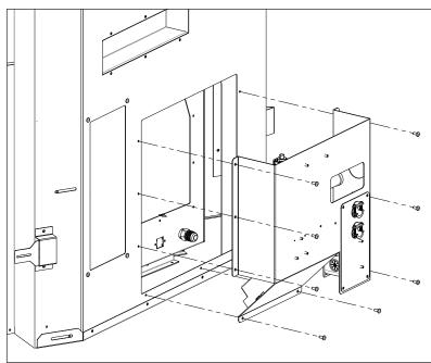
Figure 12: Component Backpack Removal
