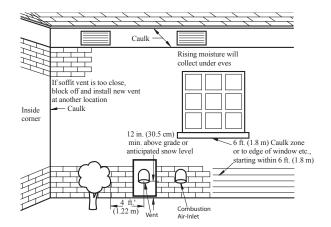
AWARNING: Moisture in the flue gas will condense as it leaves the vent terminal. In cold weather this condensate can freeze on the exterior wall, under the eaves and on surrounding objects. Some discoloration to the exterior of the building is to be expected. However, improper location or installation can result in severe damage to the structure or exterior finish of the building
