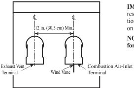
• Horizontal lengths of the vent system must slope downward a minimum of 1/8 in. per foot (10 mm per m).
