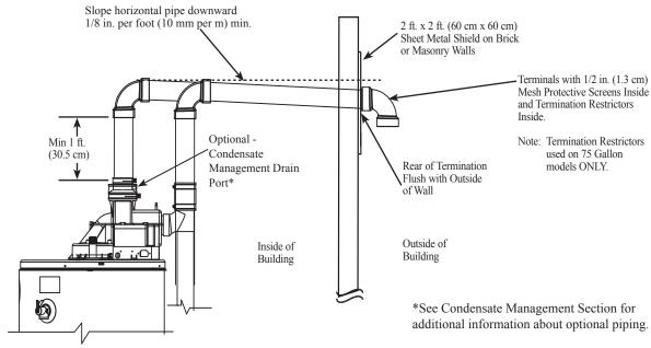
Horizontal Vent and Combustion Air-Inlet Terminal Installation
