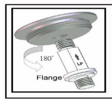
Step 3: Turn the Stem 180<sup>°</sup>so that the Flange is at The Bottom.
