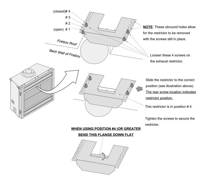
The intake restrictor is located on the back wall of the firebox. To adjust the restrictor, follow the steps below:
