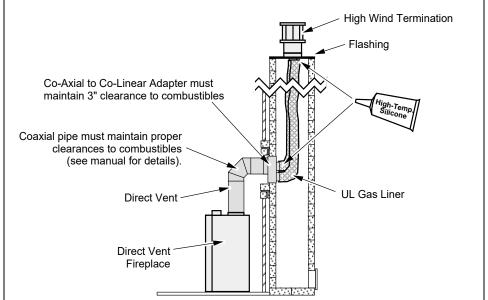
This appliance may utilize 6-5/8" diameter direct vent manufactured by Duravent (reducer may be required). The vent may be adapted to utilize an existing masonry fireplace using the Duravent Masonry Chimney Conversion Kit (part # 46DVA-KCT). The vent must be installed following all directions included with the vent and those listed below:
