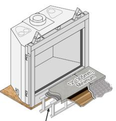
If installed near carpet on other combustible flooring, the fireplace must be raised so the base of the unit is above the carpet surface or flooring material.
