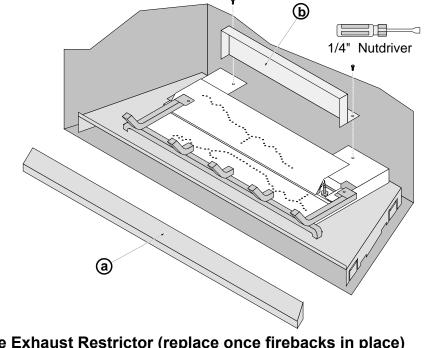
Remove the Exhaust Restrictor (replace once firebacks in place)
