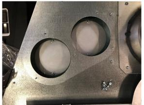
5. Use snips or diagonal cutters to snip the tab on the 2 knockouts located on the cover plate (relocated to the right side in the previous step). Press on the far side away from the tap to pop the edge of the knockout up. Grab on to the knockout with pliers and bend it back and forth until the remaining tabs break free. Repeat this step with the second knockout on the cover plate. Discard the knockouts.
