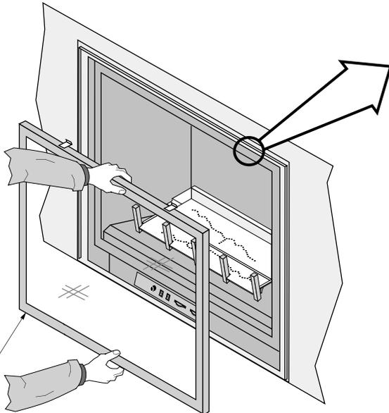
**b** Lift the glass frame up and pull it forward to remove.
