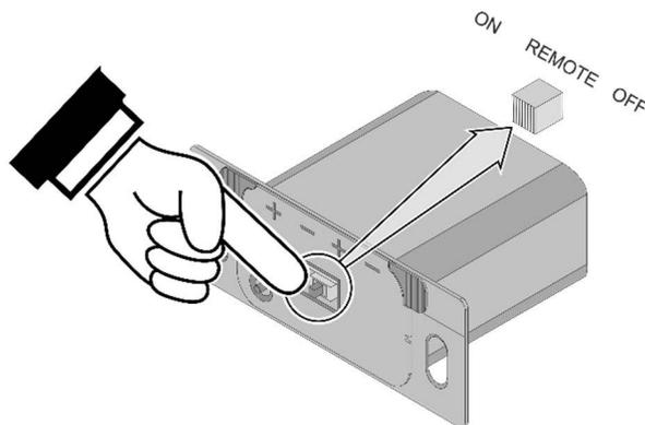
**NOTE:** When the battery holder switch is turned to ON or OFF, the mode settings (Flame Height, Comfort Control) will remain in the same state as before the switch was moved (i.e.: the IFC “remembers” the last setting). If you wish to adjust the mode settings use the transmitter mode button to adjust the settings (see “Mode Controls” on page 13). The thermostat and burner on/off operating functions will not work on the transmitter.
