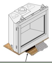
If installed near carpet on other combustible flooring, the fireplace must be raised so the base of the unit is above the carpet surface or flooring material.
