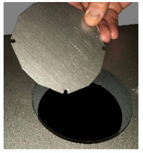
10 You will need to remove a third cover plate on each side. Remove the 2 screws holding the cover plate in place. Reach in and remove the cover plate. You may discard this plate.
