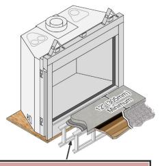
If the fireplace will be installed so that it is recessed into the floor and the combustible flooring will be on the same level as the noncombustible hearth, the hearth must be entirely constructed of non-combustible material (framing, sheeting, and finish material). For this type of installation, the hearth must be a minimum of 12" (305mm) deep and must not extend above the fireplace opening.
