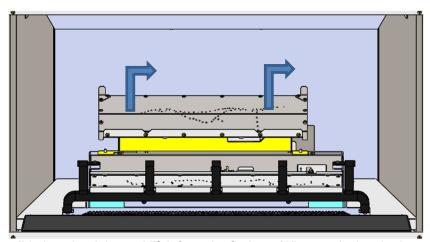
Lift the front burner, slide it to the right, and lift it from the firebox. When replacing the burner make sure it is properly located.
