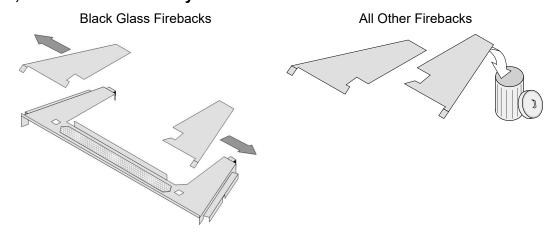
Rear Air Deflector (behind the rear log) Must be Removed (replace after firebacks in place)
