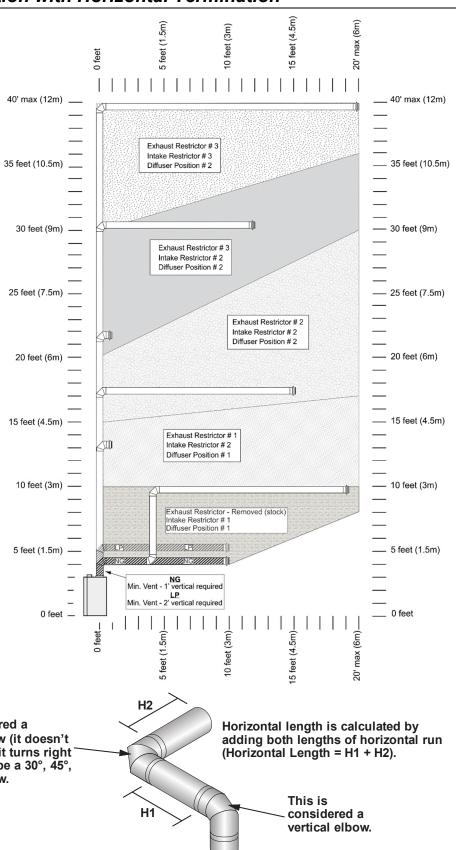
This is considered a horizontal elbow (it doesn't matter whether it turns right or left). It may be a 30°, 45°, 60°, or 90° elbow.
