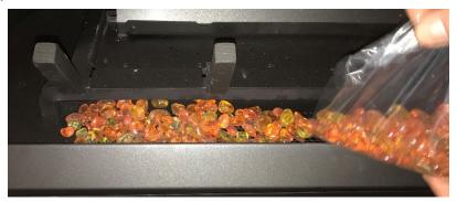
• Lightly dress the ember glass with black touch-up paint (we recommend Stove Bright®). Check the appearance with the lights on and add additional paint, as needed, for a realistic glowing ember appearance.
