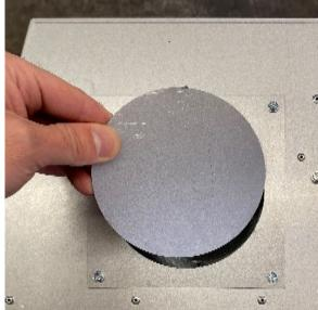
Under each knock out plate, you will find a cover plate held in place with (2) 1/4" screws. Use a nut driver or drill with an extension to remove the (2) screws. Reach in and remove the cover
