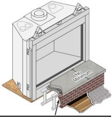
A hearth may be installed in front of the fireplace and may cover the lower portion of the fireplace up to, but not above the fireplace opening. If a hearth is installed in this manner, the hearth must be entirely constructed of noncombustible material (framing, sheeting, and finish material). There is not minimum hearth depth requirement for this type of installation and combustible flooring may be installed up to the front of the hearth as shown above.
