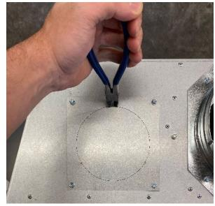
Grab on to the knockout with pliers and bend it back and forth until the remaining tabs break free.
