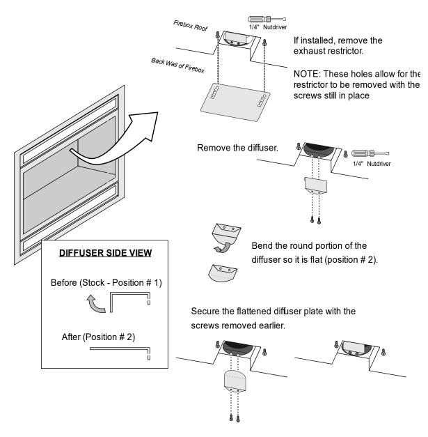
If needed, Replace the exhaust restrictor (see "Exhaust Restrictor Adjustment" for details).
