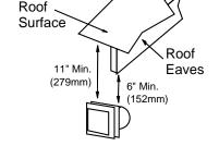
E Minimum 11" (279mm) clearance below unventilated soffits or roof surfaces
