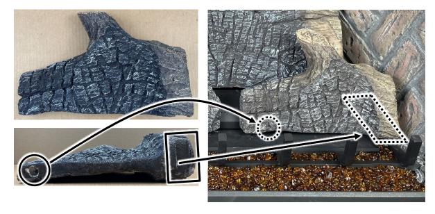
7. Place log #4 as shown below. There are (2) notches on the bottom of the log that help orient the log to the log grate. The charred end of the log should be to the left and be angled toward the center of the burner. The cut end should rest slightly forward of the log grate between the (2) right fingers of the log grate (see below). Make sure burner holes are not obstructed.
