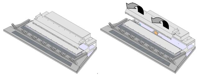
3. Remove the front burner. Lift up on the burner and remove it from the firebox (see below).
