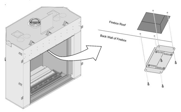
To adjust the restrictor to a different position, loosen the 4 screws holding the adjuster plates in place. Slide the to the correct notch (each notch is sequential, position # 1 through 5). Tighten the screws to secure the adjuster plates.
