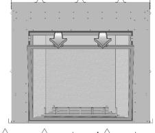
d) The screen rests against (2) tabs on the upper sides of the fireplace opening. Slide the tabs behind the front wall of the fireplace to make room for the removal of the glass assembly.
