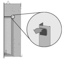
b) Lift the bottom trip straight up. When the trim is above the front edge of the fireplace opening, remove it from the fireplace and set it aside.
