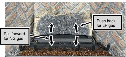
5. Place log #2 on the front burner. The notch on the bottom left of the log rests on the grate. The hole on the right end of the log rests on the locating pin just left of the center of the burner. Push the log backward until it is in contact with the rear burner.
