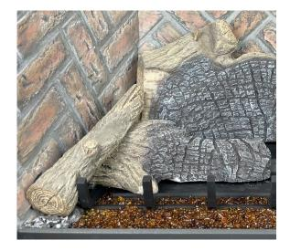
9. Place log #6 as shown below. There is a flat spot on log #5 and log #2 for log #6 to rest on. Place the hole in the bottom of the charred end of log #6 onto the left locating pin on the top of log #2
