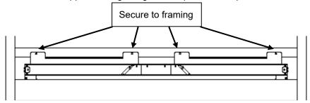
6 Re-attach the two rear mounting brackets (removed in step 6) to the bottom of the convection manifold. Leave the screws loose so the brackets can be positioned to the back of the chase. Secure the brackets to the chase using screws (not included). Tighten the screws securing the brackets to the manifold.
