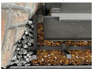
4. Place log #1 as shown below. The two slots on the bottom of the log sit over the pin on the burner. With the rear log in place, **push it back if using LP gas or pull it forward if using NG gas.**
