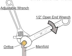
**(b)** Apply thread sealant to the LP orifices prior to installation. Use the chart below to identify the correct orifices.
