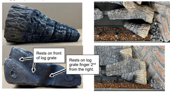
8. Place log #5 as shown below. There is a notch on the lower right of the log that rests against the leftmost fireplace grate finger. The upper portion of the log rests on a flat spot on the top of log #2.
