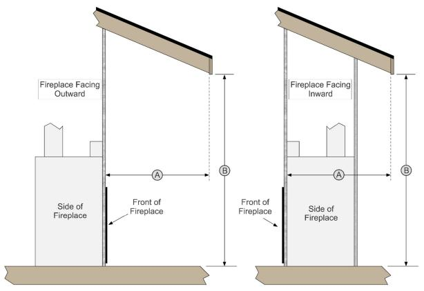
The overhang (A) must extend at least 1/2 the roofline height (B). Height is measured from the base of the fireplace.
