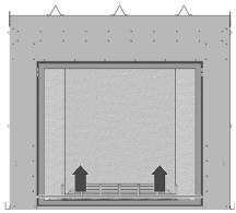
c) Tip the barrier screen outward and remove the screen.
