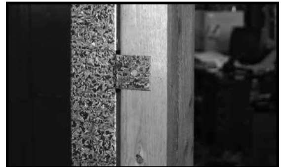
Figure 19: Framing tabs bent out.
