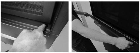
2. Lift up on the barrier screen assembly until the top brackets are clear of the tabs on the glass frame assembly. Direct the top edge of the barrier screen forward. Lift the bottom tabs out of the brackets on the bottom of the glass frame assembly and remove the barrier screen from the fireplace.
