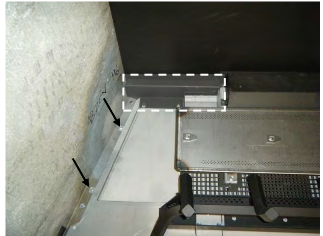
Step Five: Reinstall Liner Supports and Screws.
