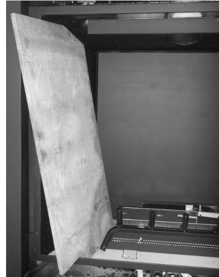
Step Three: Tilt and slide left and right Side Liners into place.
