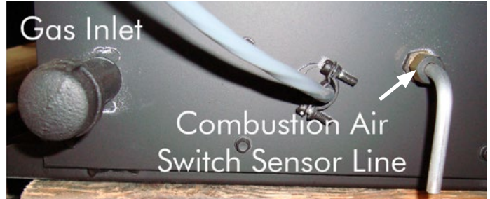
Figure 9.b.b Identifying the Gas Inlet and Combustion Air Switch Sensor Line
