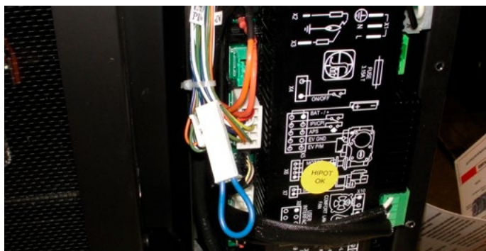
Figure 19.c Connectez le câble de raccordement CPI
