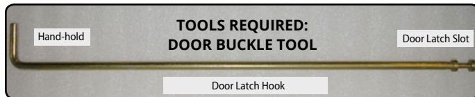
Figure 20.a Door buckle Tool
