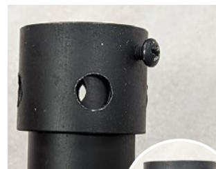
Figure 13.c Adjusting the orifice
