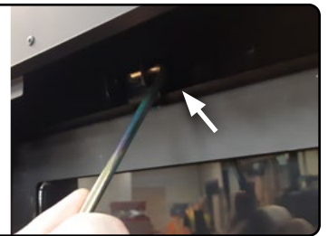
Figure 21.d Pull door latches
