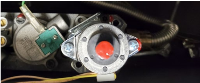
Figure 13.eee LP pressure regulator on a Full Load
