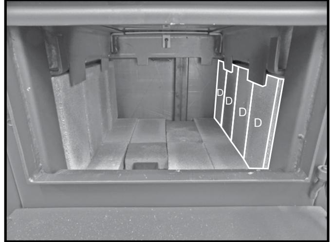
Figure 17: Bricks on right side wall in place.
