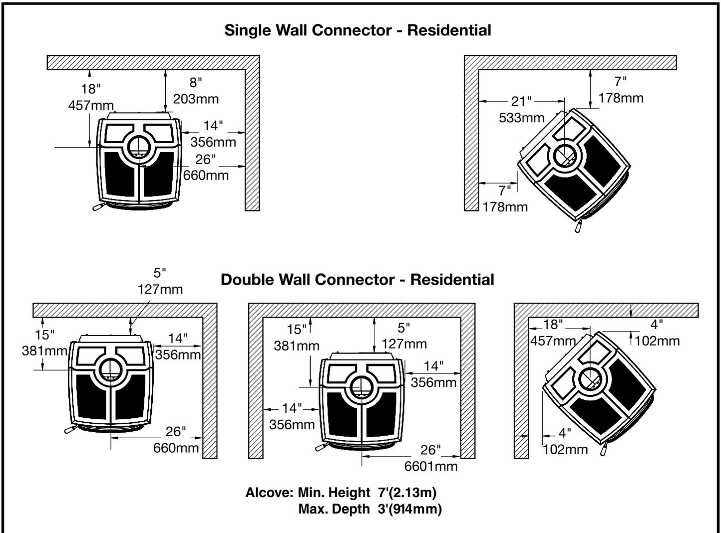
Figure 4: T5 Minimum clearances.
