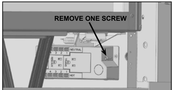
Figure 8.3 Junction Box Detail - COSMO32-IFT-B
