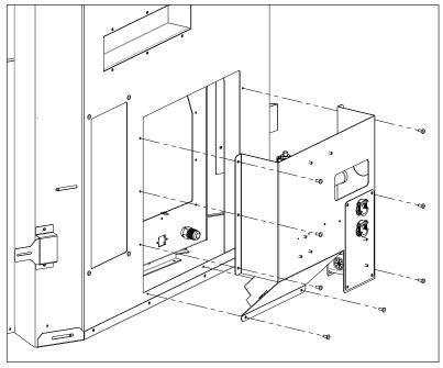
Figure 13: Component Backpack Removal
