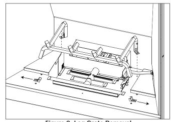
Figure 9: Log Grate Removal
