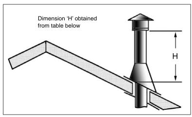
Figure 68: Height of Vertical Termination; Reference Table 8
