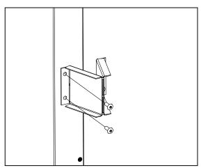
Figure 29: Rear Standoff Install
