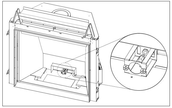
Figure 22: Orifice Location
