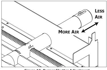
Figure 12: Burner Shutter Adjustment
