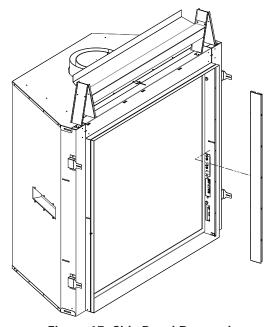
Figure 17: Side Panel Removal
