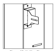
Figure 27: Nailing Flange Assembled
