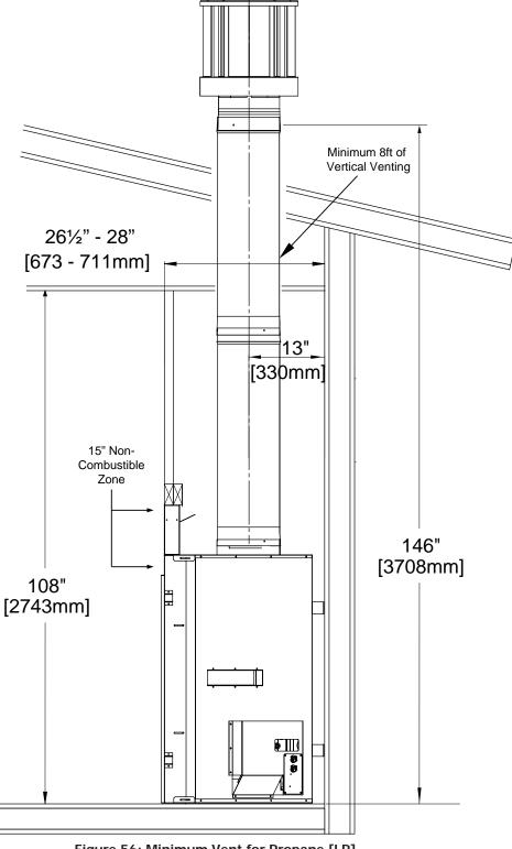
Figure 56: Minimum Vent for Propane [LP]
