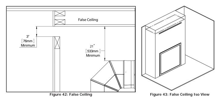
**Option 2: Open Chase (built-out installations) -** This could be considered the most discreet option when considering the CSS. The chase must be constructed in a way that stops short of the ceiling, leaving it totally vented above. Minimum framing dimensions must be followed when constructing this option and not to deviated from them when using combustible materials. Consider **Optional 3: Valance** to work in conjunction with this option.
