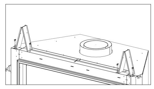
Figure 31: Top Standoff Install
