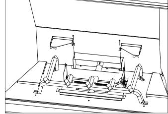
Figure 8: Log Mount Removal
