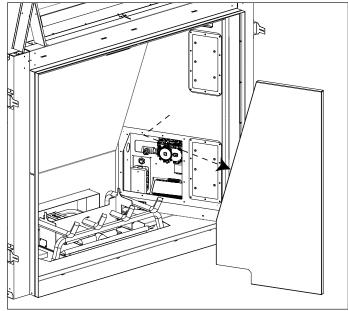
Figure 20: Right Liner Removal
