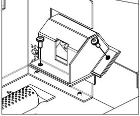
Figure 23: Pilot Shield Removal
