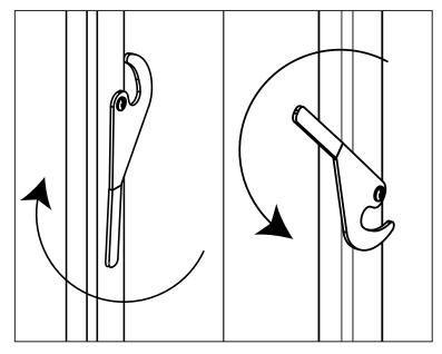
Figure 7: Door Hook Unlock (Left) and Lock (Right)
