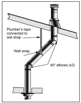
Figure 69: Multi-Story Vent Pipe Installation
