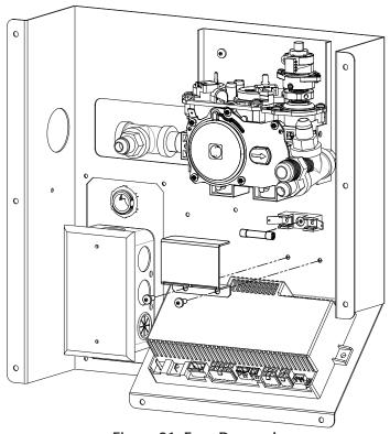
Figure 21: Fuse Removal
