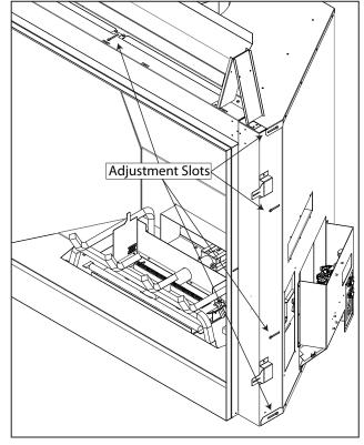
Figure 36: Framing Depth Adjustment
