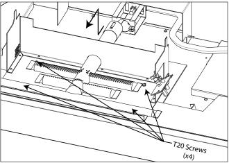
Figure 11: Log Burner Removal
