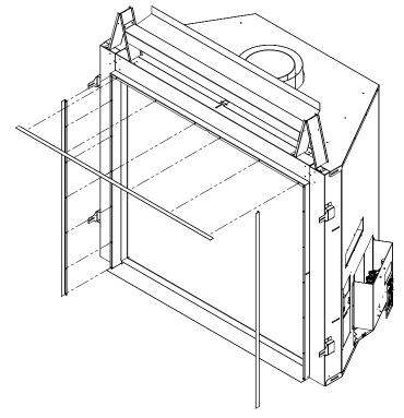
Figure 33: Finishing Edge Removal / Installation
