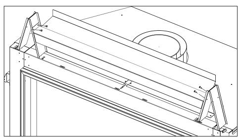
Figure 32: Top Standoff Support Install
