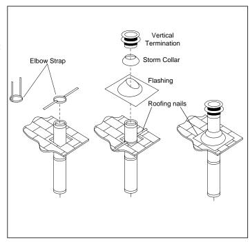
Figure 67: Vertical Vent Termination
