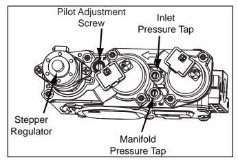
Figure 71: Fully Labeled Gas Valve.
