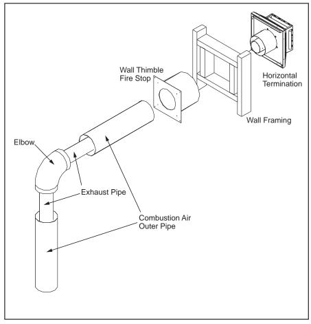
**Figure 66: Horizontal Vent Termination**
