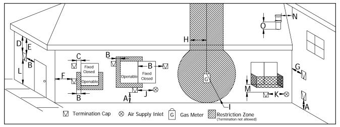
Figure 60: Vent Termination Restrictions, refer to Table 2
