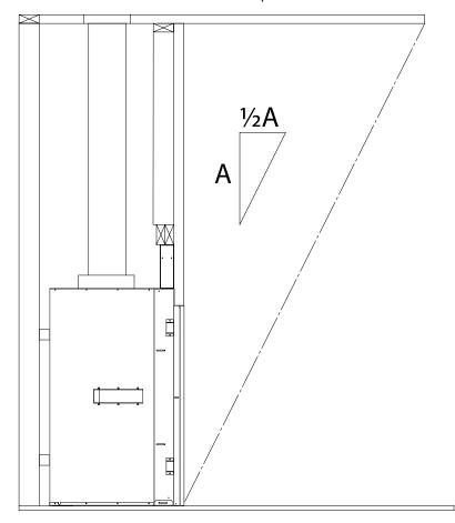
Figure 52: Overhang Depth Requirements
