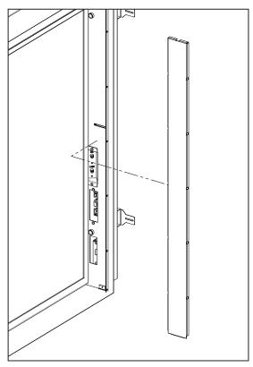
Figure 35: Side Cover Removal
