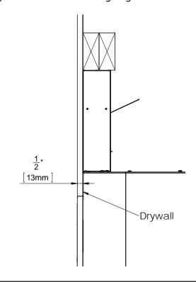
**Standard Thick Facing Install:** By adjusting the cabinet back, **non-combustible** material may be layered on top of the supplied Noncombustible board. Supplied board not needed for thick **non-combustible** finishes like rock.
