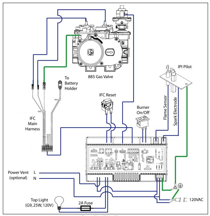
Figure 72: Wiring Diagram
