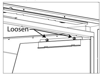
Figure 19: Liner Retainer Removal
