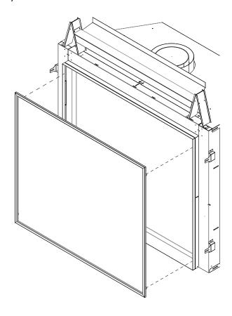
Figure 4: Safety Screen Removal
