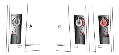
4. Connect the three cables to the three counterweights and tighten the nuts that hold them in place.
