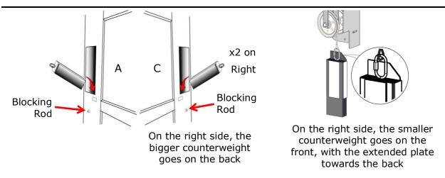
3. The counterweights will be supported by the pre-installed blocking rods. Ensure the blocking rods are in position before inserting the counterweights.
