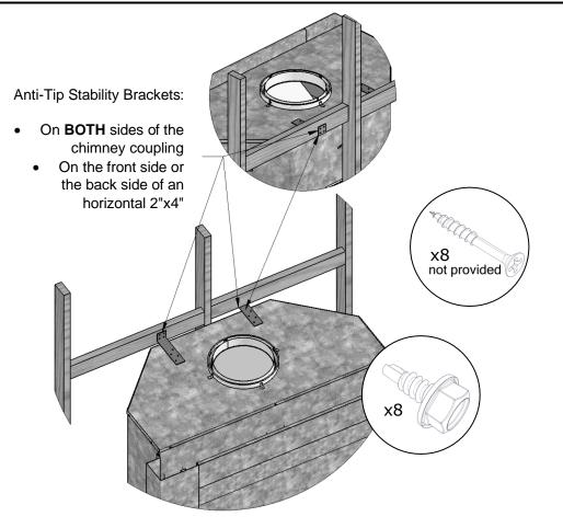
FIGURE 9 ANTI-TIP BRACKET INSTALLATION
