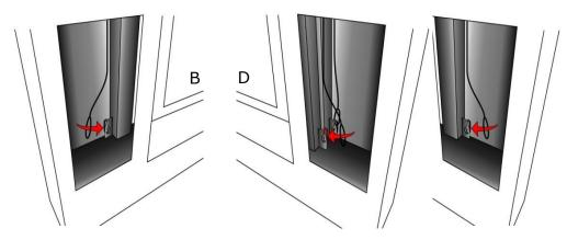
5. Connect the hanging cables to the bottom of the door left and right, and to the bottom of the firescreen at the front right.
