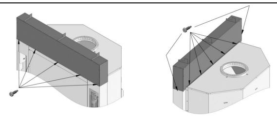
FIGURE 6 INSTALLATION OF THE TOP FINISHING COVER
