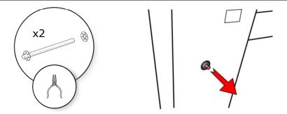
6. Using pliers, remove the caps on the back side of each blocking rod. **Do not remove the blocking rods yet.**
