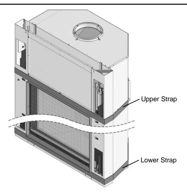
The upper strap must be located just above the upper finishing lintel.
