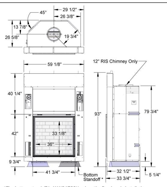
\*The bottom standoff is MANDATORY unless the fireplace is installed a on non-combustible floor (structure and surface), like a foundation over earth for example.
