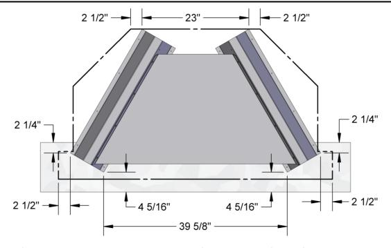
FIGURE 8 POSITIONING THE FIREPLACE BOTTOM STANDOFF AND SPARK GUARD
