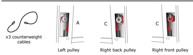
2. Start by placing the three counterweight cables through the openings A and C, and over the pulleys. Allow the cables to hang down towards the door.
