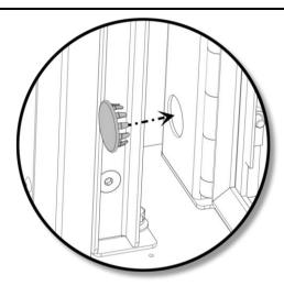
2. Locate the two door cover buttons in the manual bag and push them into the holes in the door frame.
