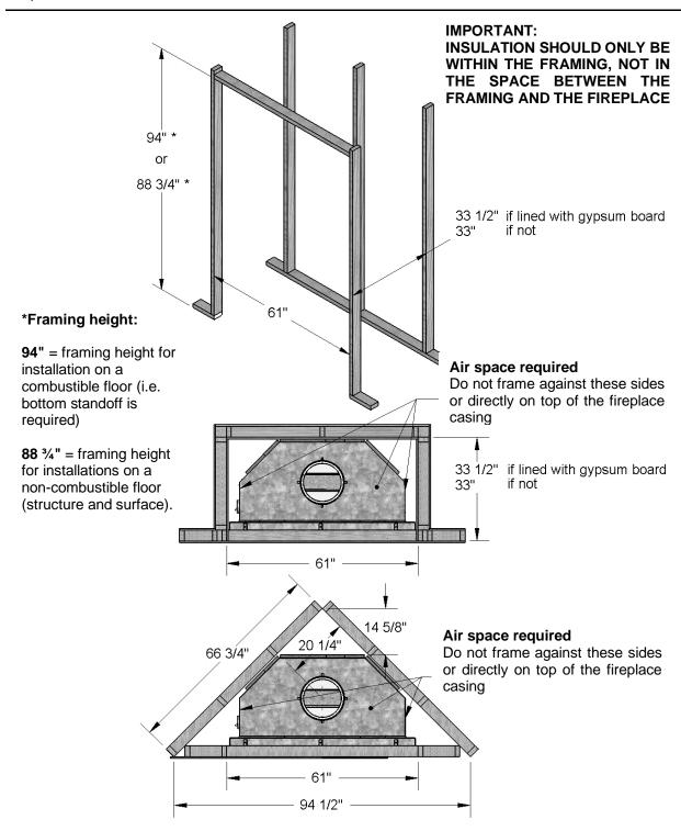
The minimal recommended framing dimensions do not take into consideration the space required for the outside air connection because the location for it and the space required are specific to your installation. Take the time to plan.
