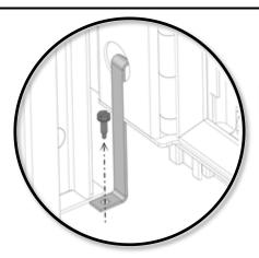
1. The guillotine glass door is held closed by two transportation blocking brackets, located at the bottom of the door on each side. Remove the ¼" hex head screws and the blocking brackets.
