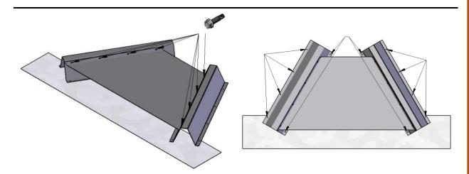
FIGURE 7 ASSEMBLING AND INSTALLING THE FIREPLACE BOTTOM STANDOFF
