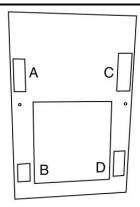
1. Openings A and C allow the insertion of the counterweights. The openings will be covered by cement board and do not have finishing metal cover plates.
