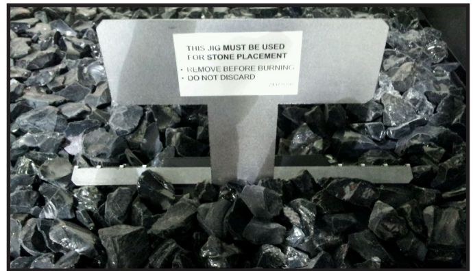
Figure 9.9 Rock Placement Jig
