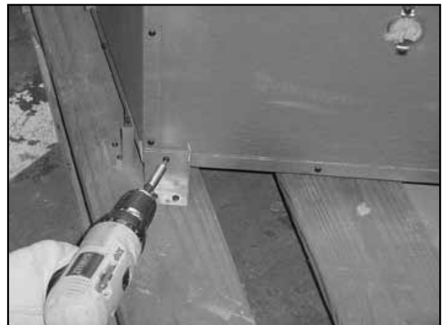
Figure 3.12 Removing Shipping Brackets
