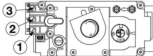
**GDS50-1 :** Disconnect the existing wires from terminals 1 and 3 (from the ON/OFF switch) and replace with the leads from the wall switch / millivolt thermostat.
