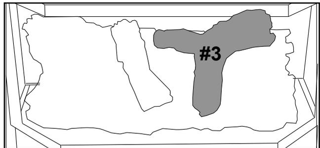
4. Align the square pegs on log #3 with the notches on the right end of the base log.
