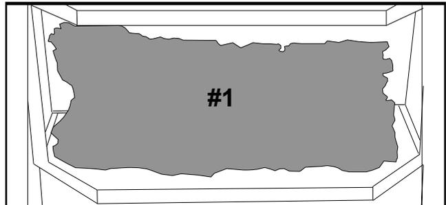
2. Place the base log #1 between the log supports, ensuring that it is pushed back against the back of the supports.
