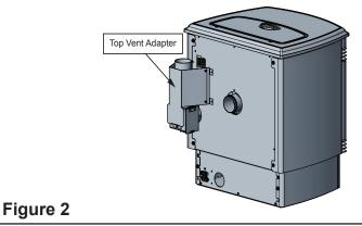
Ensuring the adapter is in the vertical position. Drill 4 holes with #26 drill bit (C3) into the back of the stove using the outer shield on the adapter (C1) as a guide. Secure using four mounting screws (C2) (Figure 3).
