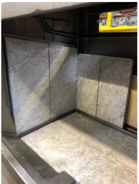
Photo 2. Left side refractory stone installed.
