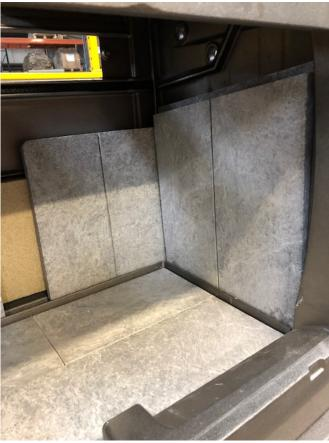
Photo 4. Right side refractory stone installed.
