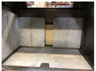
Photo 3. Right rear refractory stone installed.
