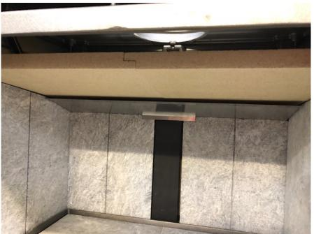
Photo 7. Vermiculite baffles installed.
