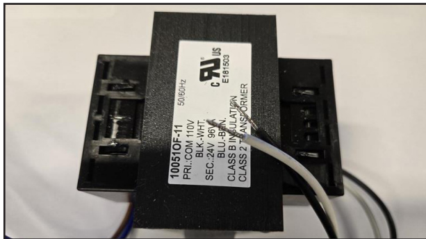
120 to 24VAC Transformer
