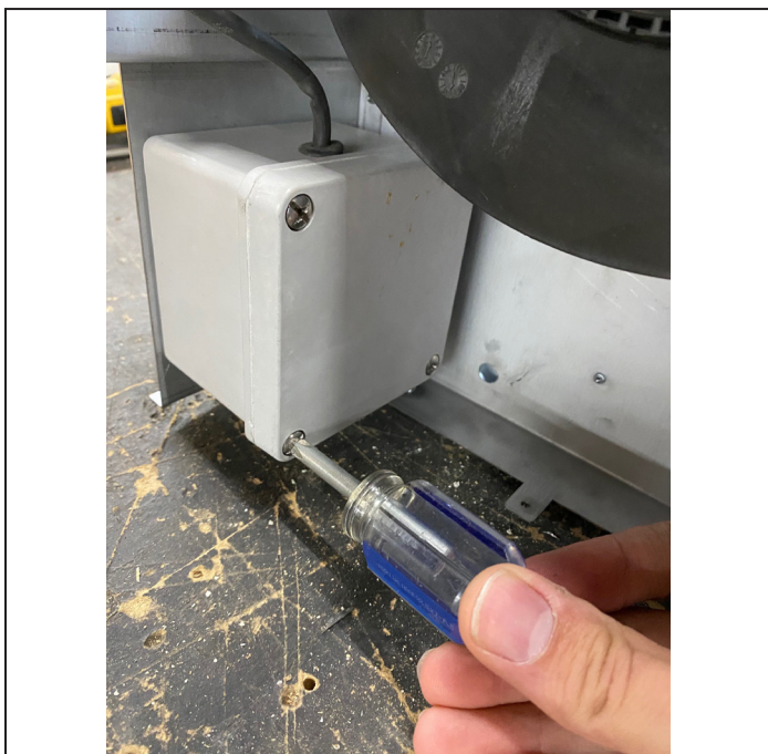
FIGURE 4.2 Remove Electrical Box Lid
